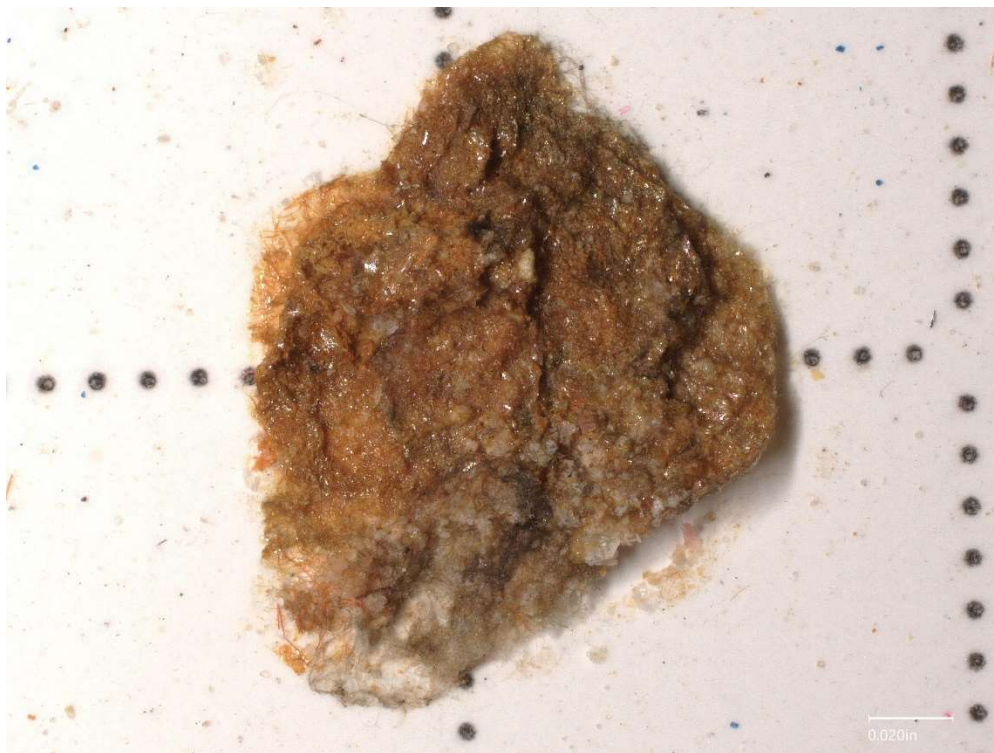
Figure 1. The debris collected from filtration during flushing of the actuator.
