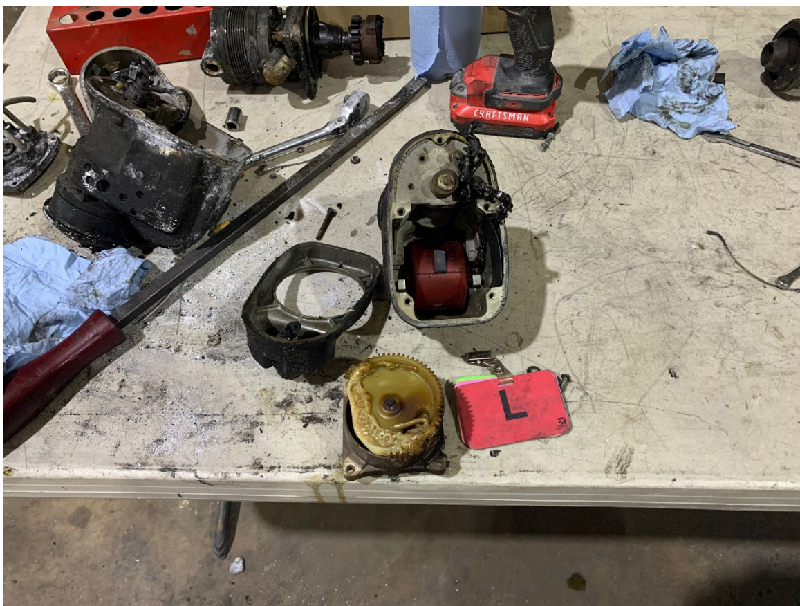
Photograph 7 - Fire damaged left magneto (NTSB Photo)
