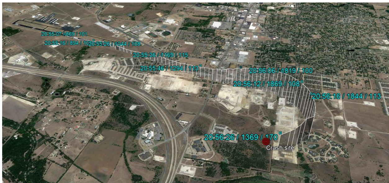
Figure 2. Google Earth image of the flight path, with selected times, msl altitude and calibrated airspeeds indicated.
