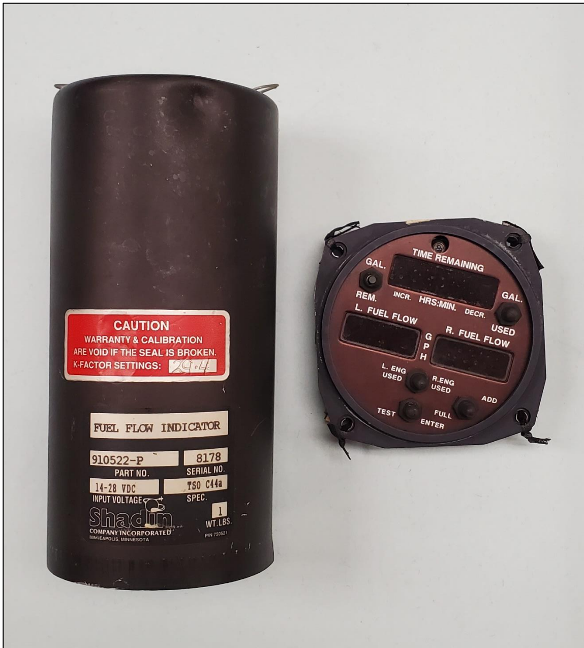
Figure 1 – Fuel Flow Indicator (as received at NTSB lab)
