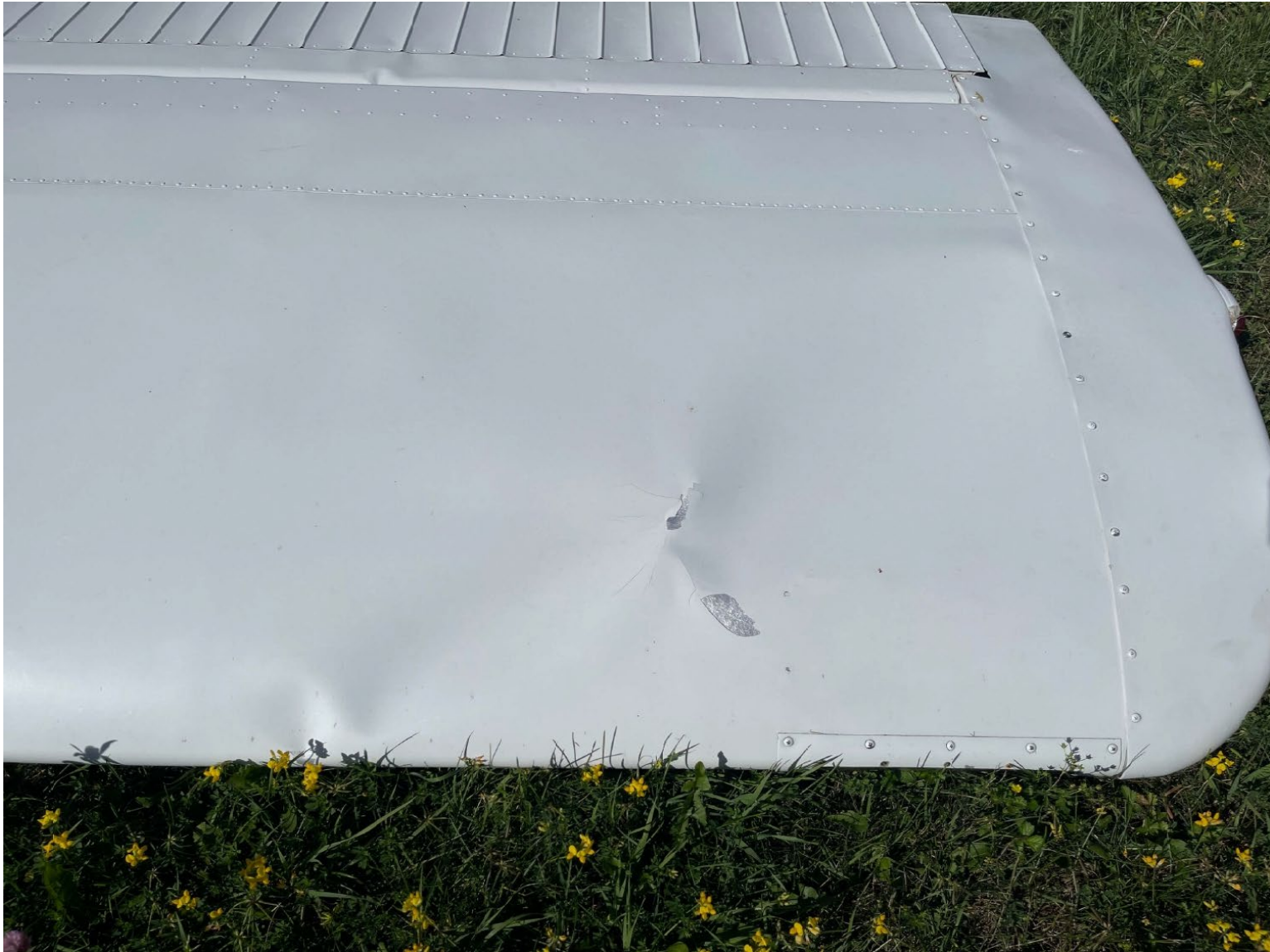
Photograph 4 - Left Wing Damage (Courtesy of Airplane Owner)
