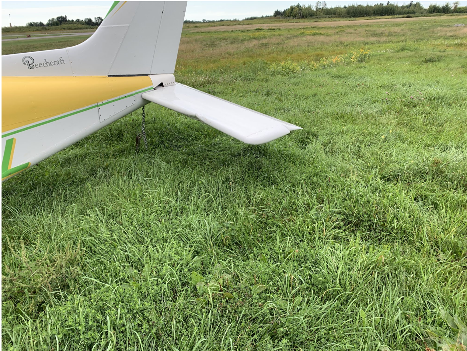
Photograph 8 - Damage to Left Side of the Stabilator (Courtesy of FAA)
