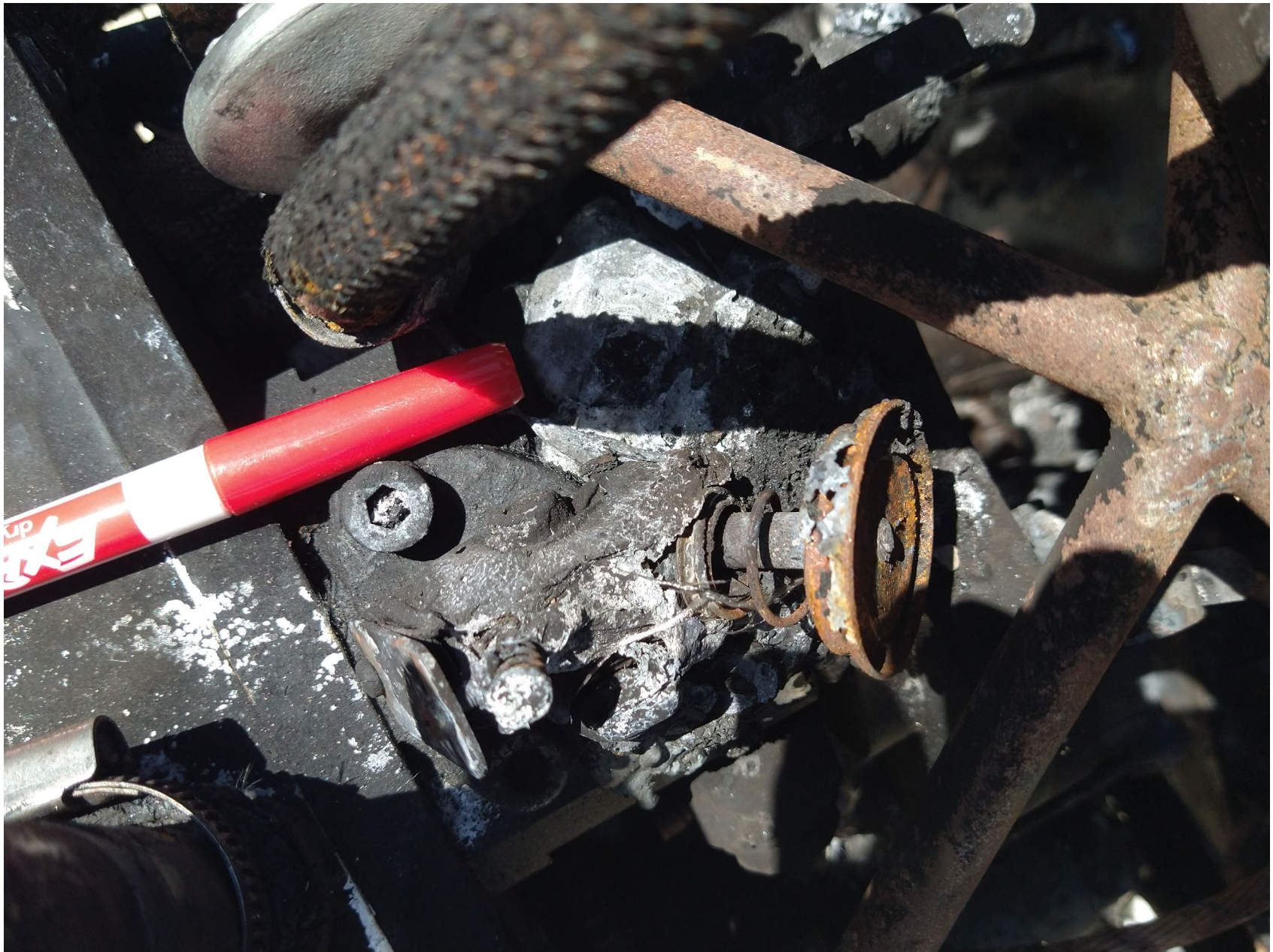
Photo 2 – Remnants of Fuel Pump (Photo from Owner)
