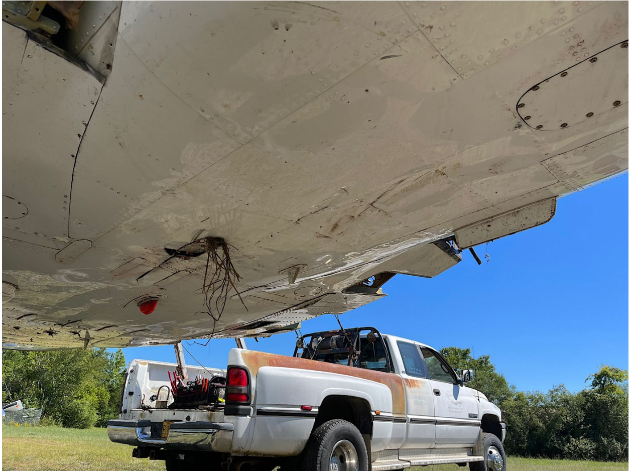
Photo 2: Fuselage Damage (Source: Dawson Aircraft)
