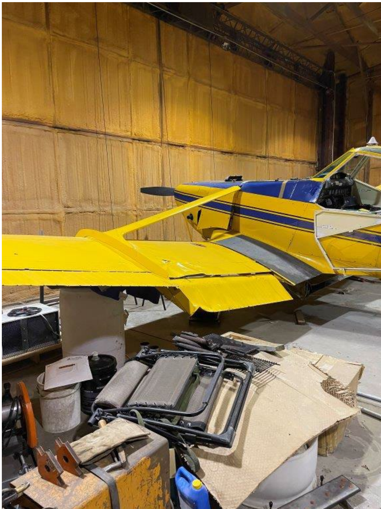
Photo 1: Left Wing Damage to N2122U (Source – Federal Aviation Administration)
