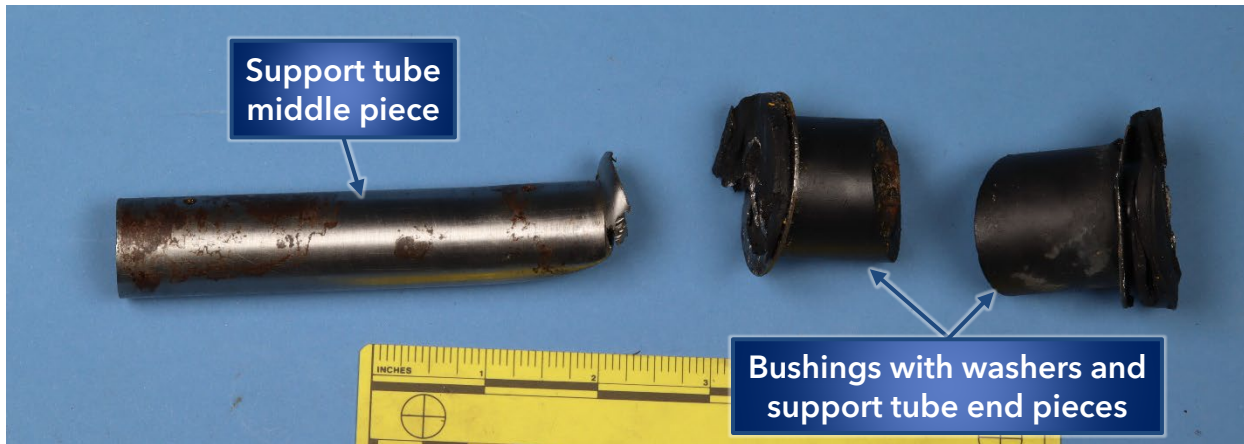
Figure 1. Support tube, washers, and bushings as received.
