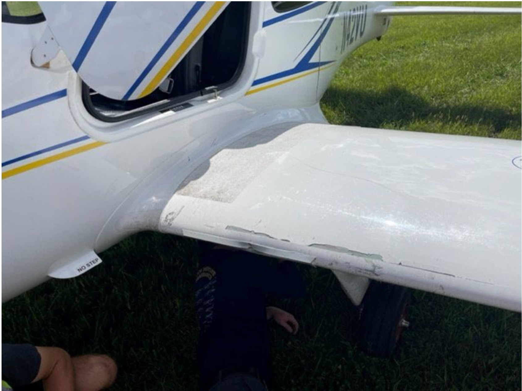
Photo 1 – Damage to left wing (Photo courtesy of FAA)
