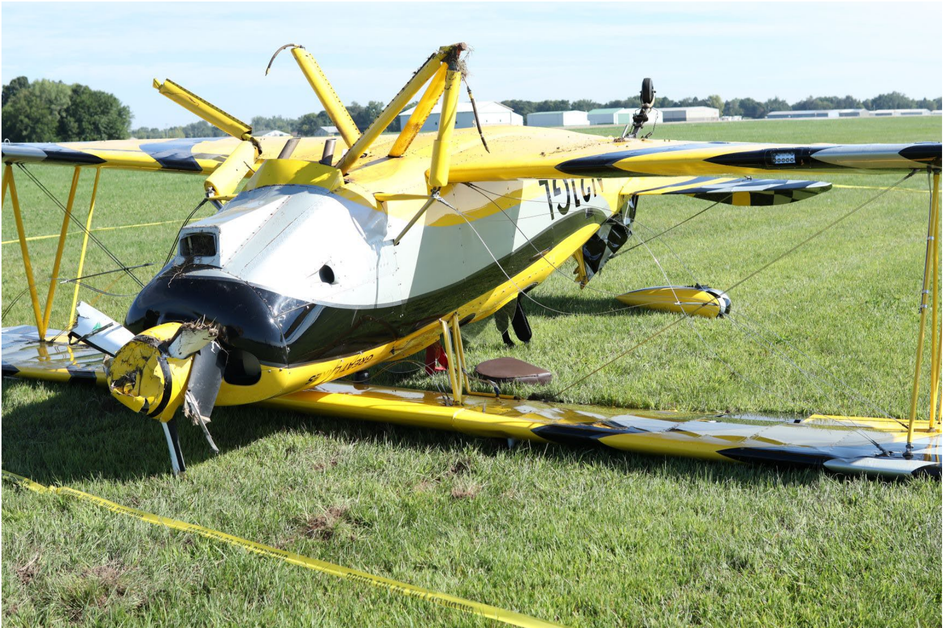
Photo 1 – Accident Airplane (photograph provided by FAA)
