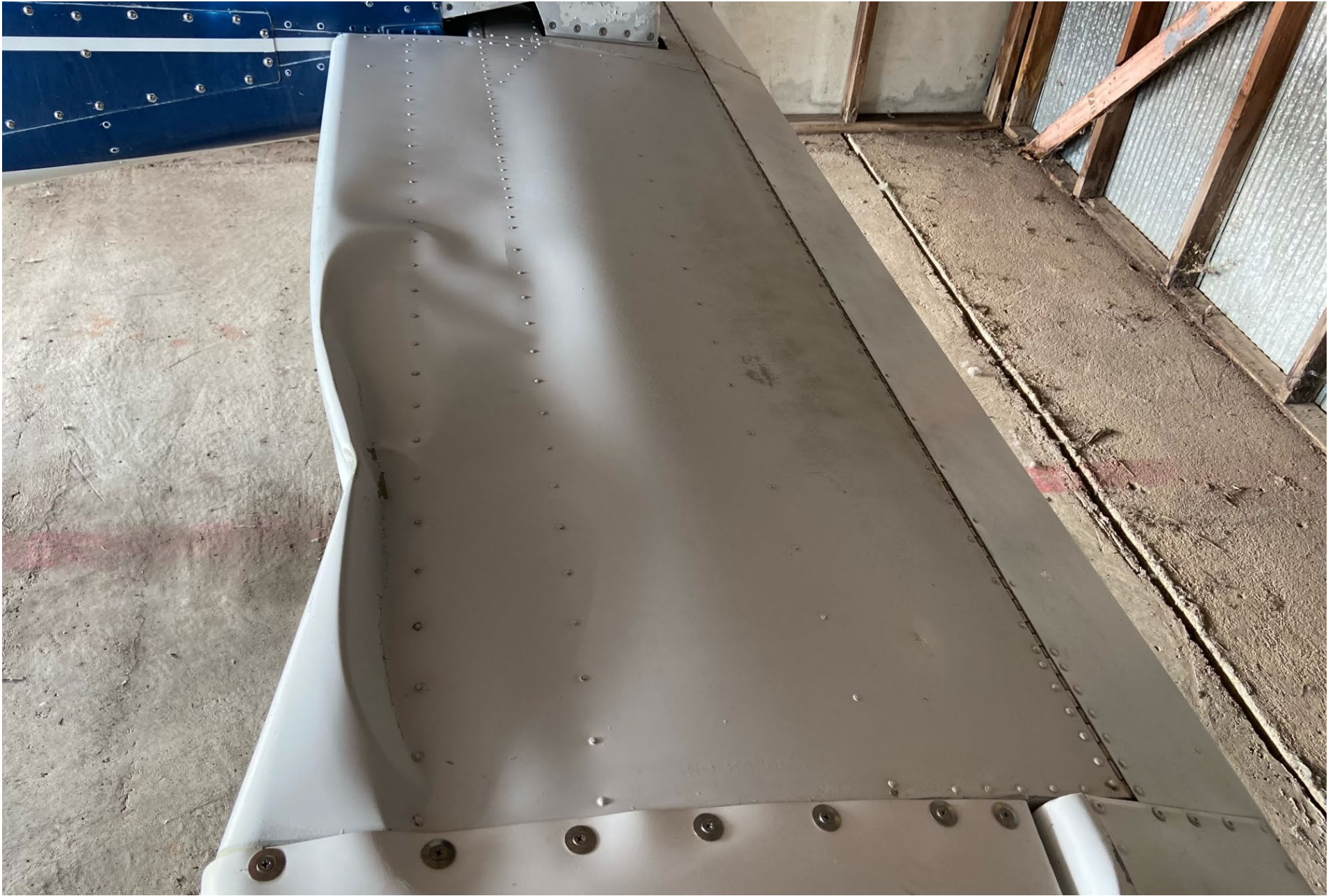
Photo 1 – Stabilator Damage (Courtesy of Federal Aviation Administration) FAA
