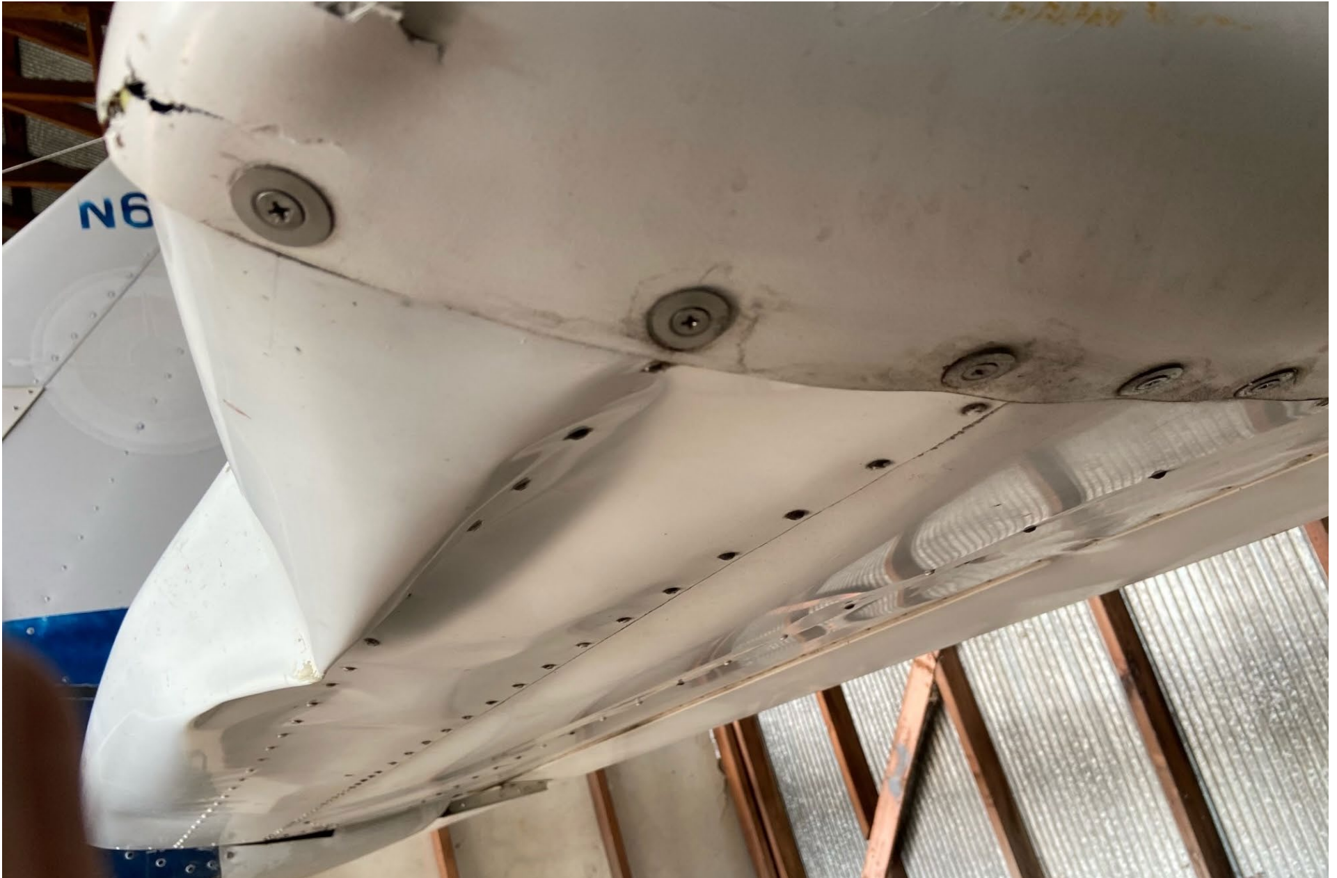
Photo 2 – Stabilator Damage (Courtesy of Federal Aviation Administration) FAA
