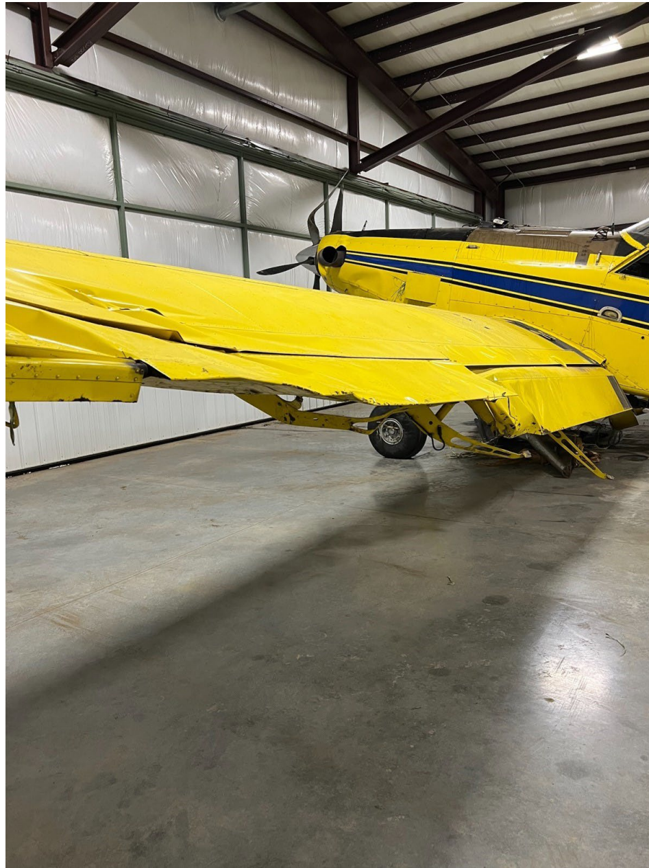
Photo 2 – Closeup of Substantial Damage to Left Wing
