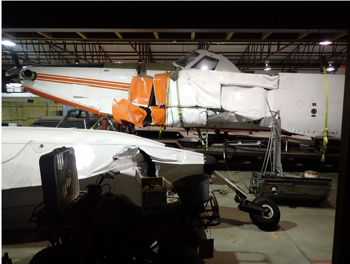
Photograph 2 - Right Wing Damage (Courtesy of FAA)
