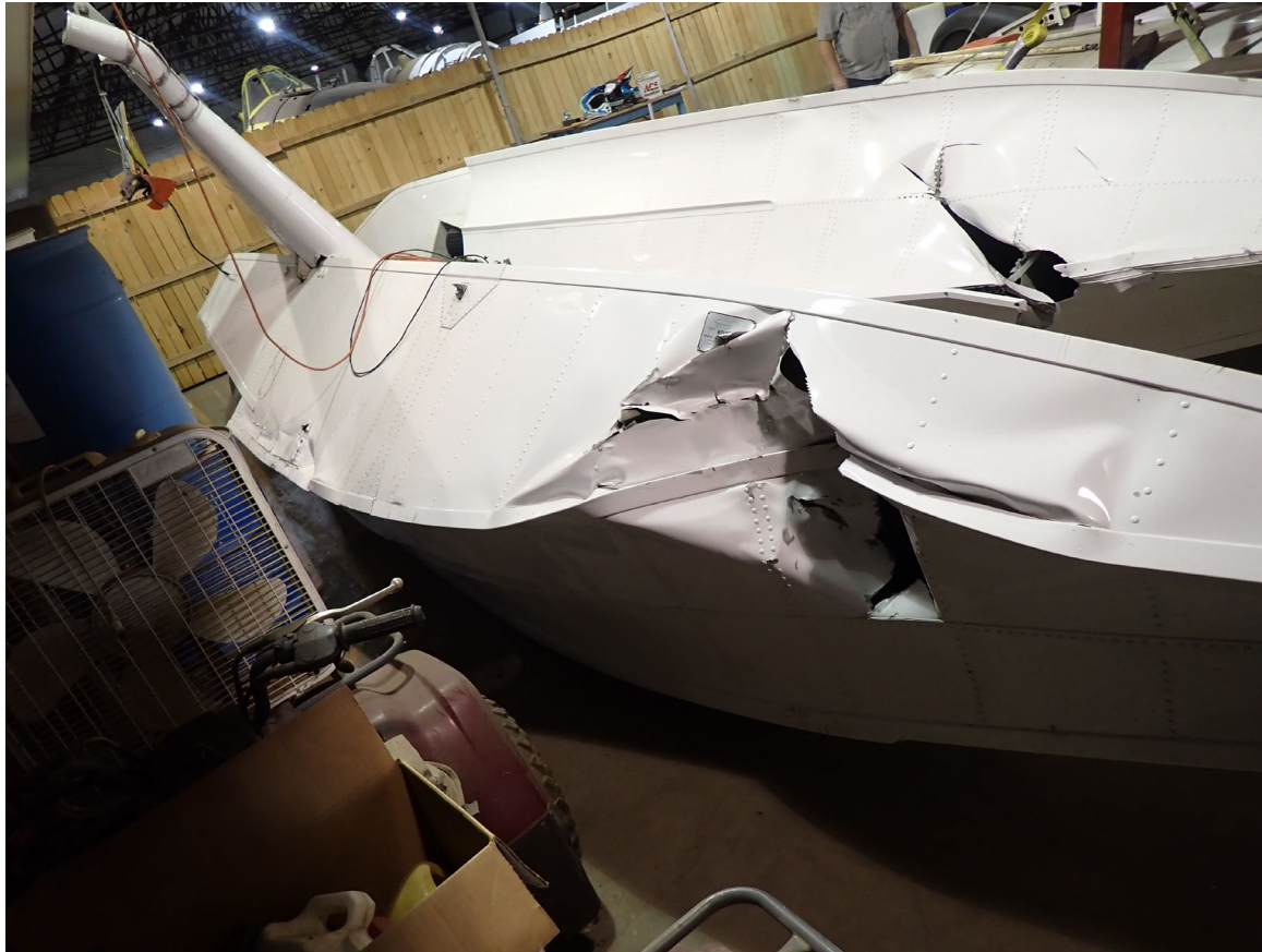
Photograph 4 - Float Damage (Courtesy of FAA)
