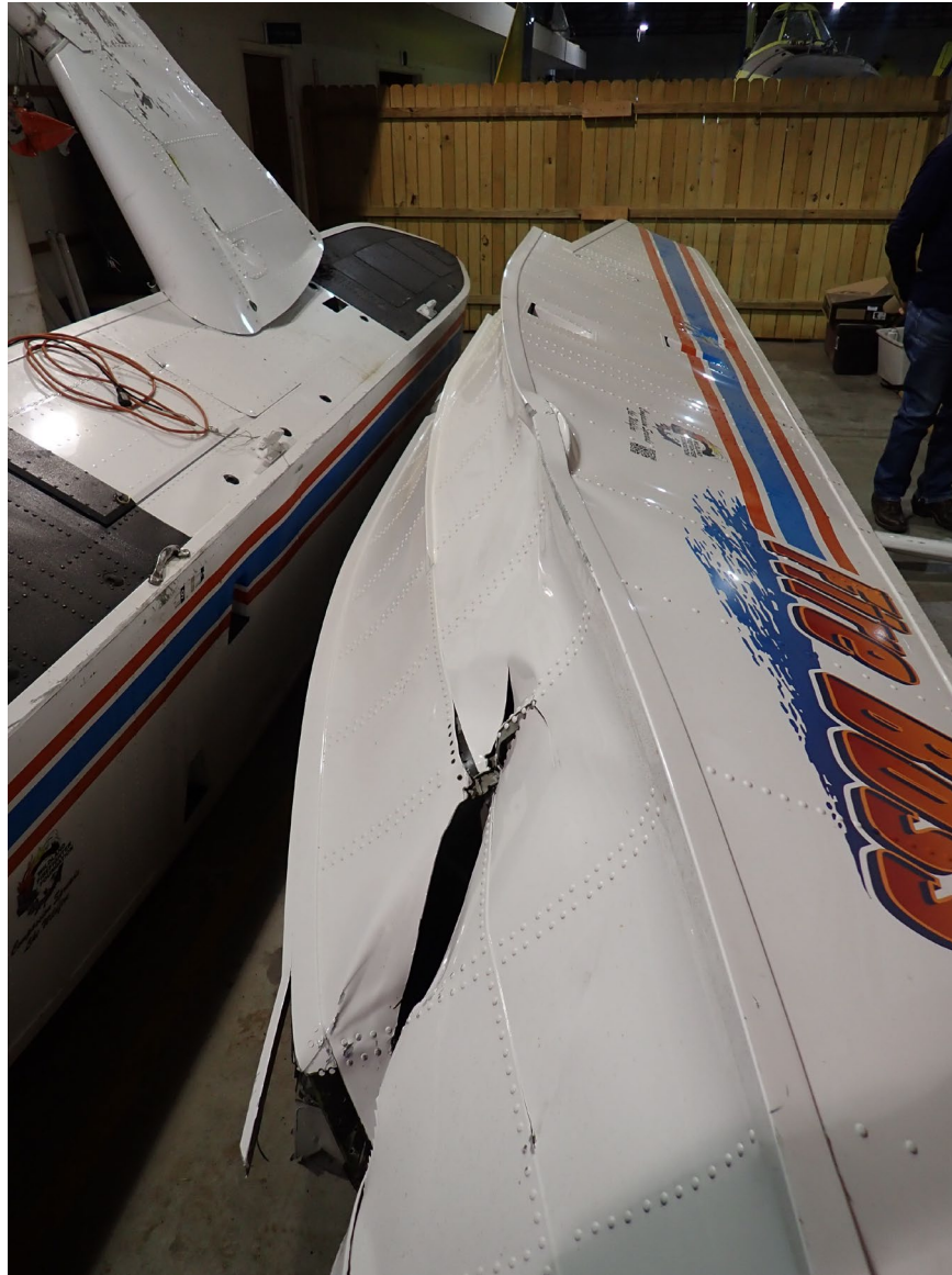
Photograph 5 - Left Float Damage (Courtesy of FAA)
