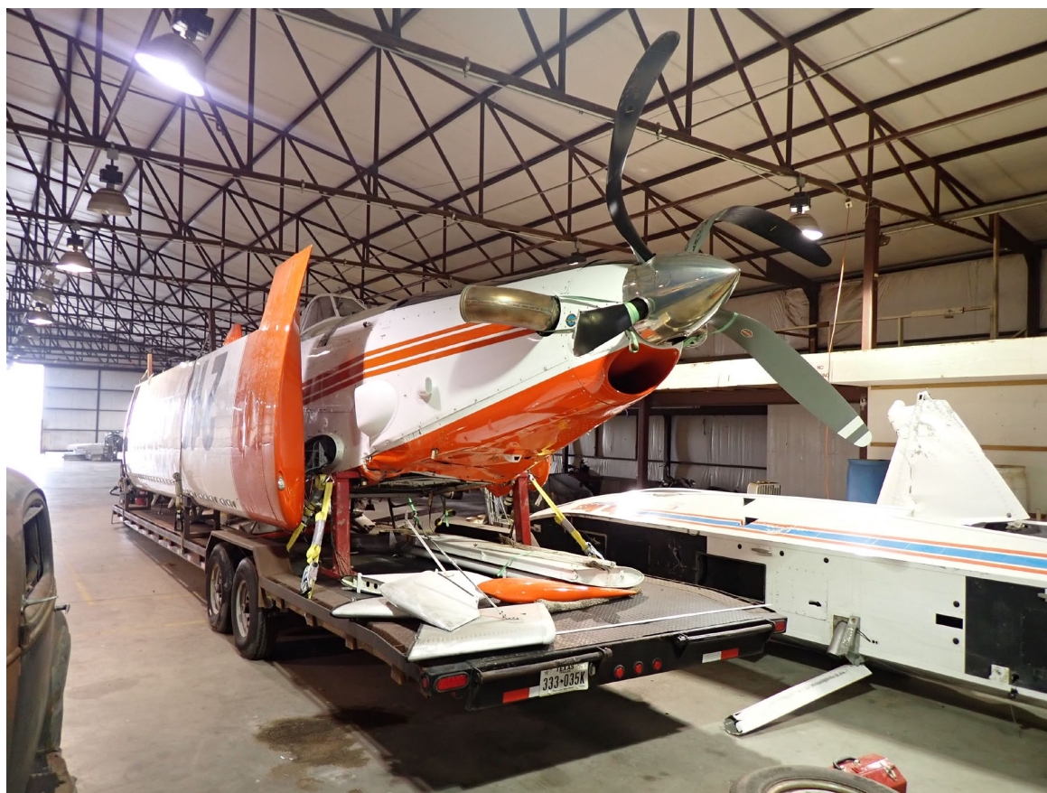
Photograph 1 - Propeller Damage (Courtesy of FAA)
