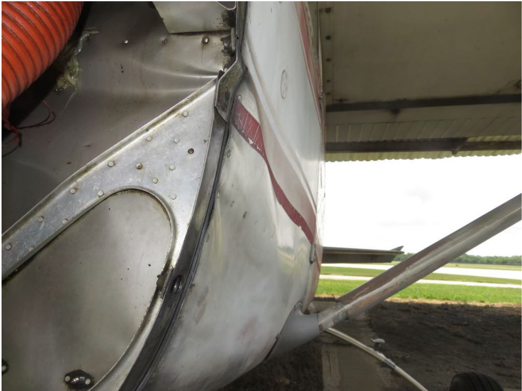
Photo 1 – Fuselage and firewall damage (Courtesy of airplane owner)
