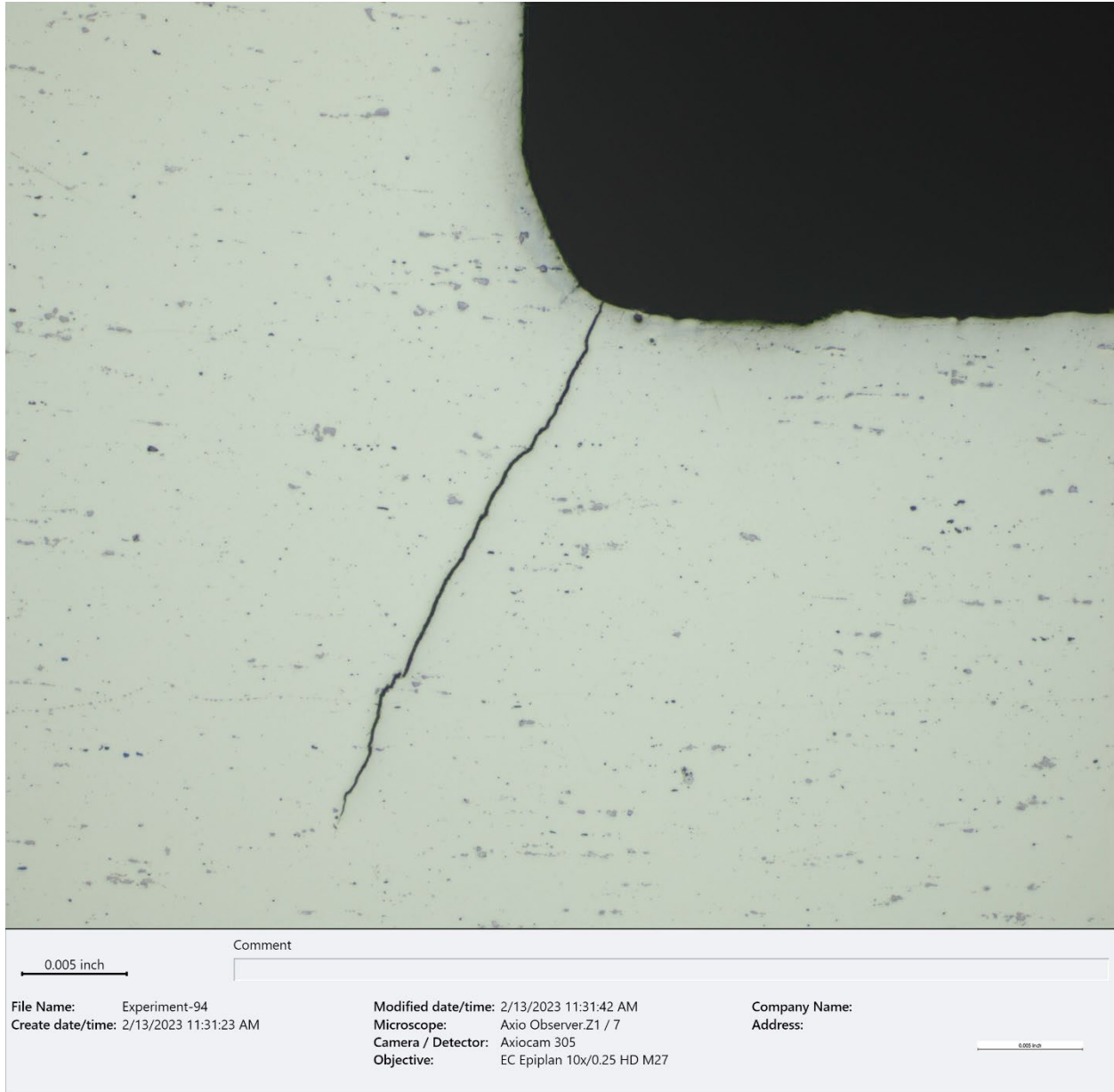
Figure 23. BF optical metallograph showing a closer view of the left corner crack from Figure 22 (~100X, as polished).
