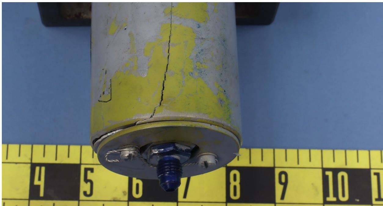
Figure 5. The longitudinal crack on the actuator housing, emanating from the circumferential crack (opposite the view in Figure 4a).
