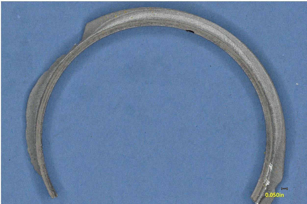
Figure 11. Montage of magnified images of the crack face of the circumferential crack, showing indications of progressive cracking.
