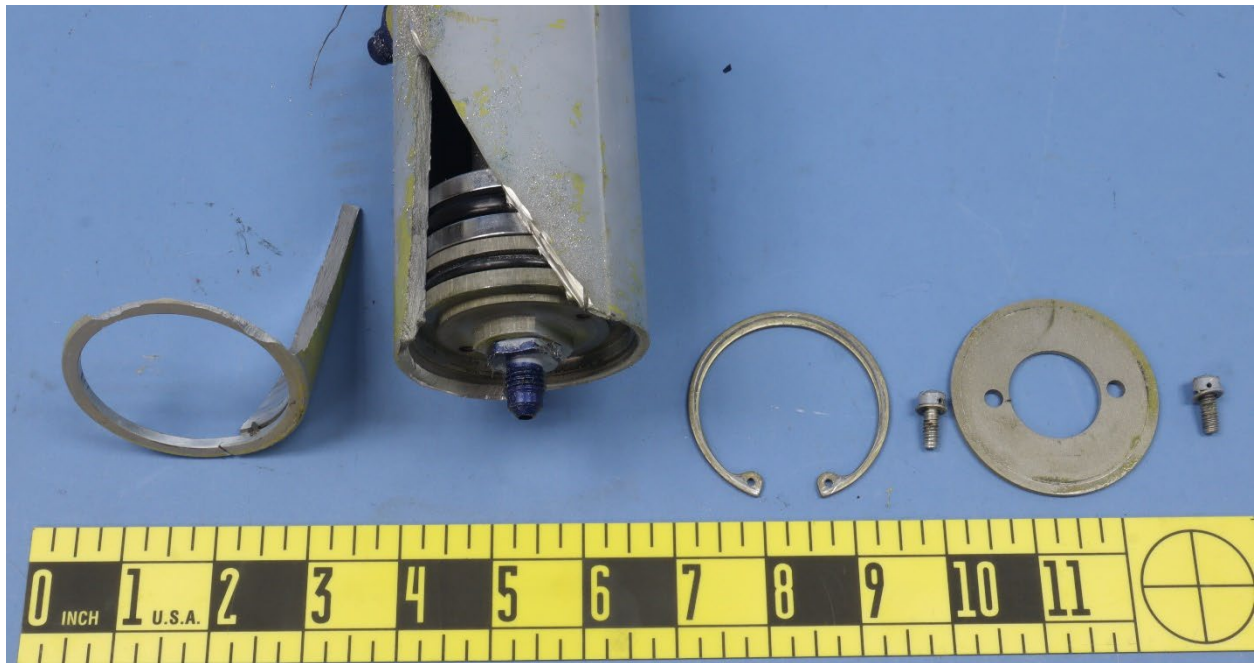
Figure 8. The cracked end of the actuator pictured in Figure 7a, after sectioning and removal of the cracked regions of the housing barrel.
