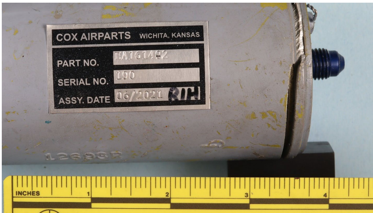
Figure 3. View of the markings on the housing barrel of the actuator, with the circumferential crack on the right.
