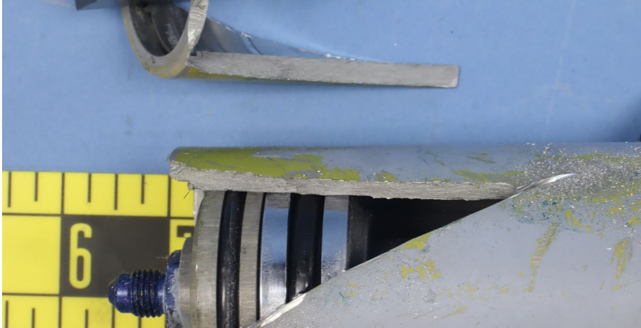
Figure 10. Mating faces of the longitudinal crack, after sectioning to open the crack faces.
