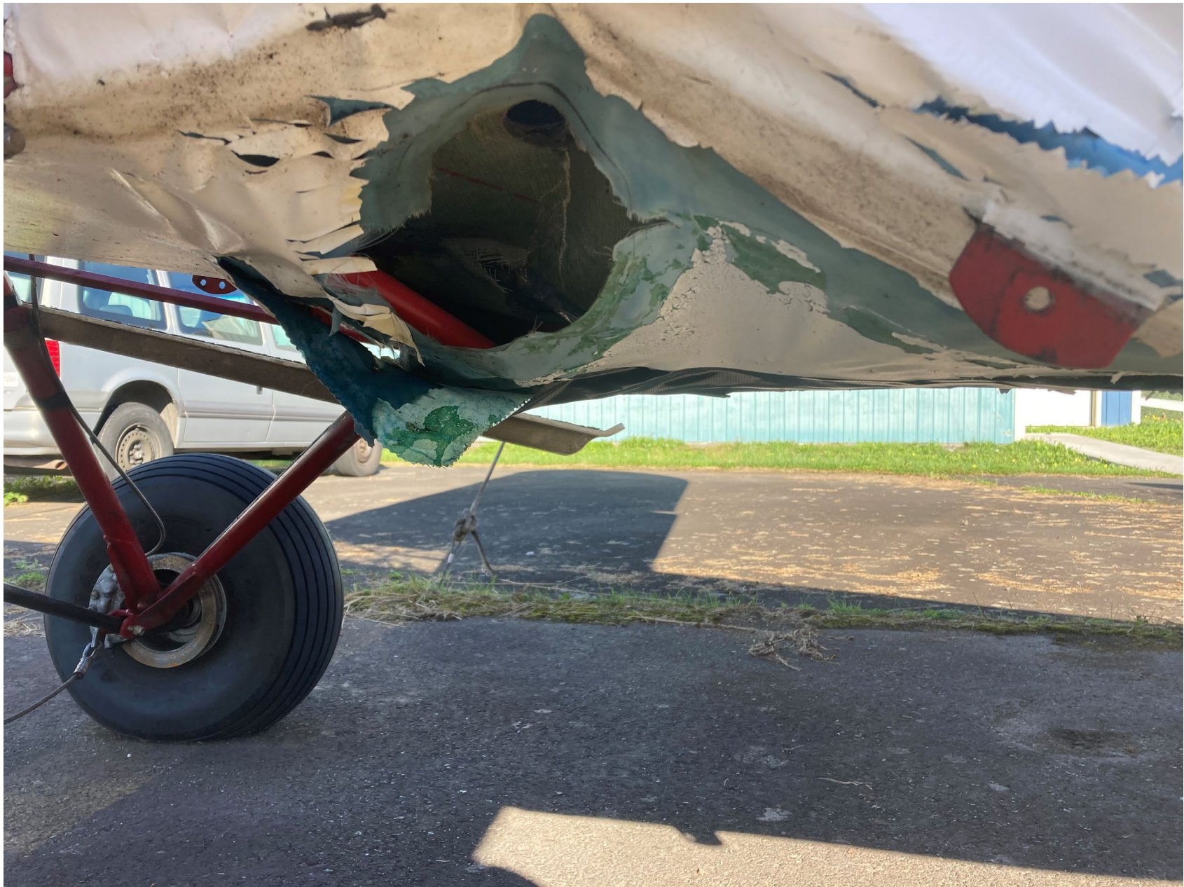
Photo 1 – Damage to the main landing gear – Courtesy of FAA (Federal Aviation Administration)
