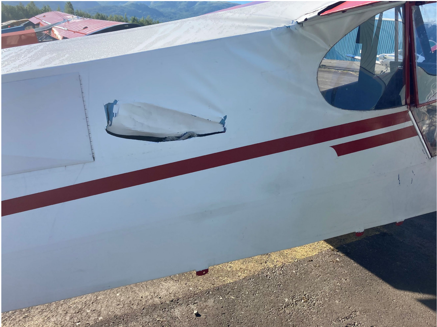
Photo 2 – Fuselage Damage to the right side – Courtesy of FAA
