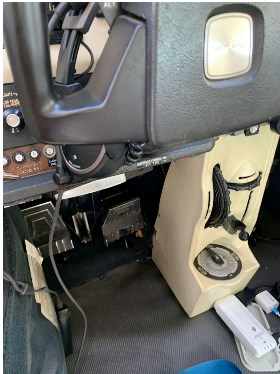
Photo 2 – Wrinkled Floor of Airplane (Provided by FAA)
