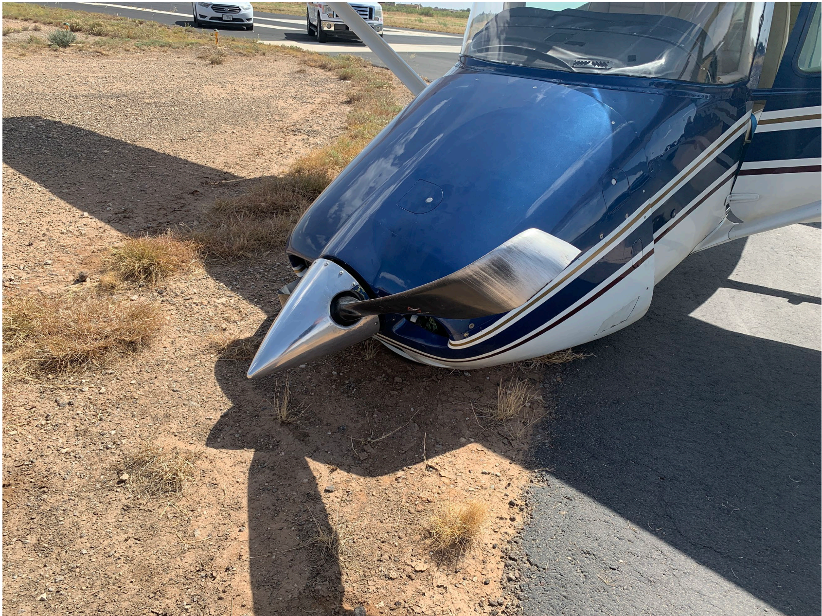
Photo 1 – Airplane with Bent Propeller and Collapsed Nose Gear (Provided by FAA)
