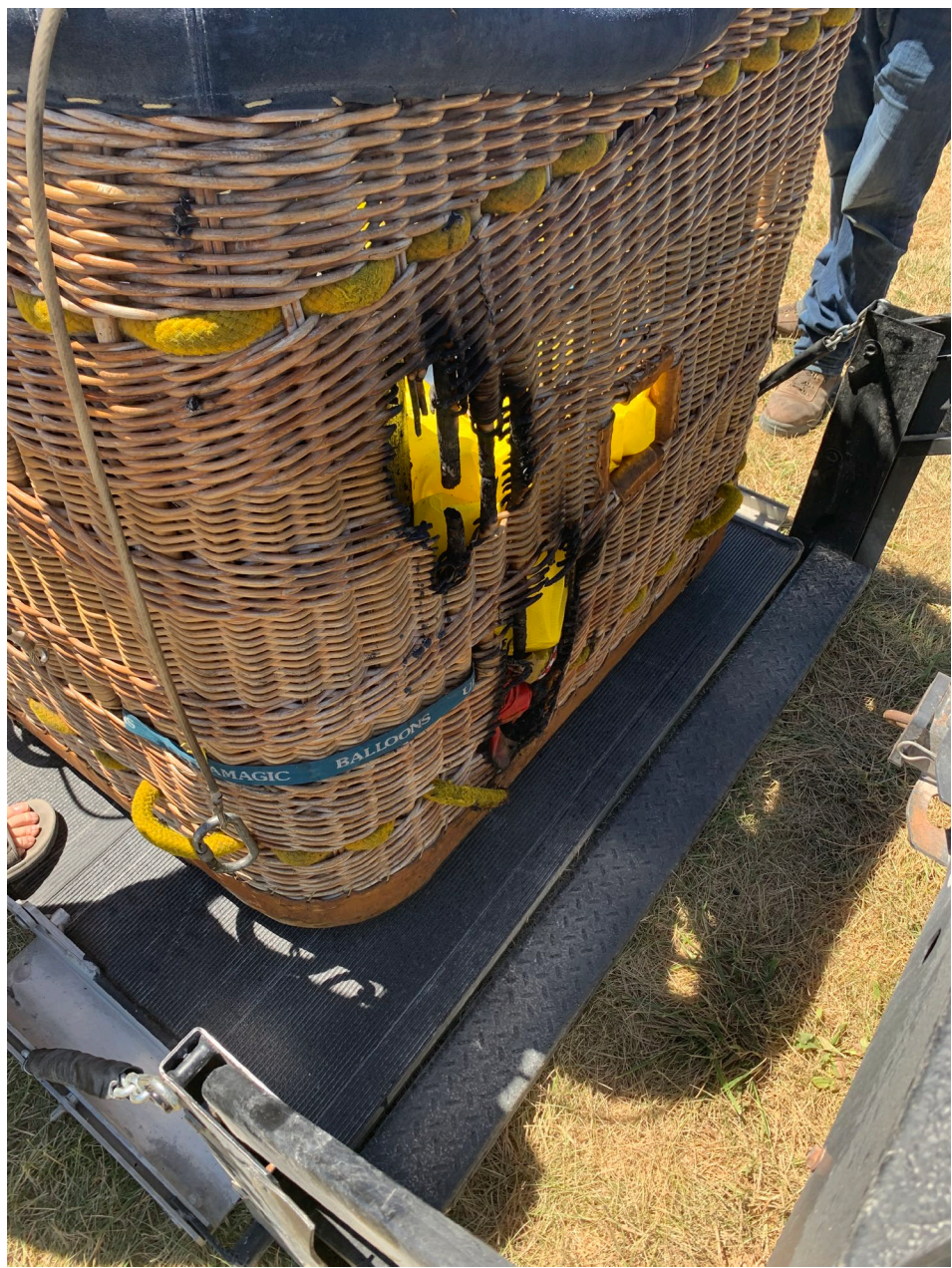
Accident Balloon / Burned holes in basket – (Photo provided by FAA)
