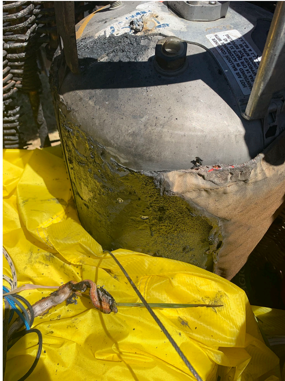
Accident Balloon / Burned propane tank – (Photo provided by FAA)
