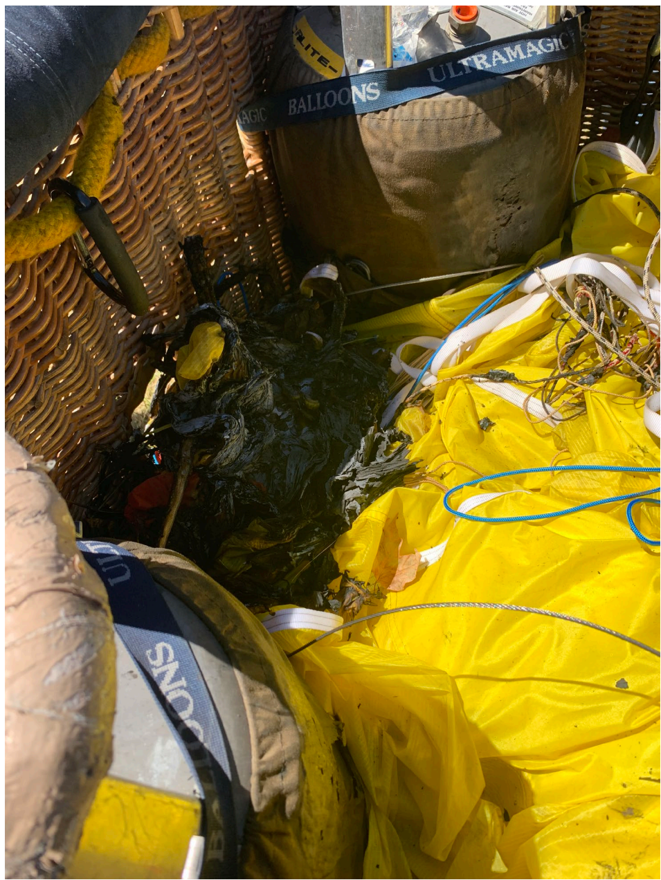
Accident Balloon / Burned Envelope – (Photo provided by FAA)
