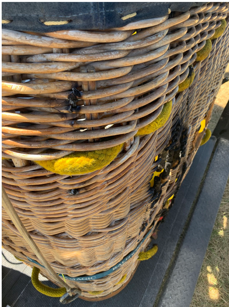
Accident Balloon / Close-up of burned holes in basket – (Photo provided by FAA)
