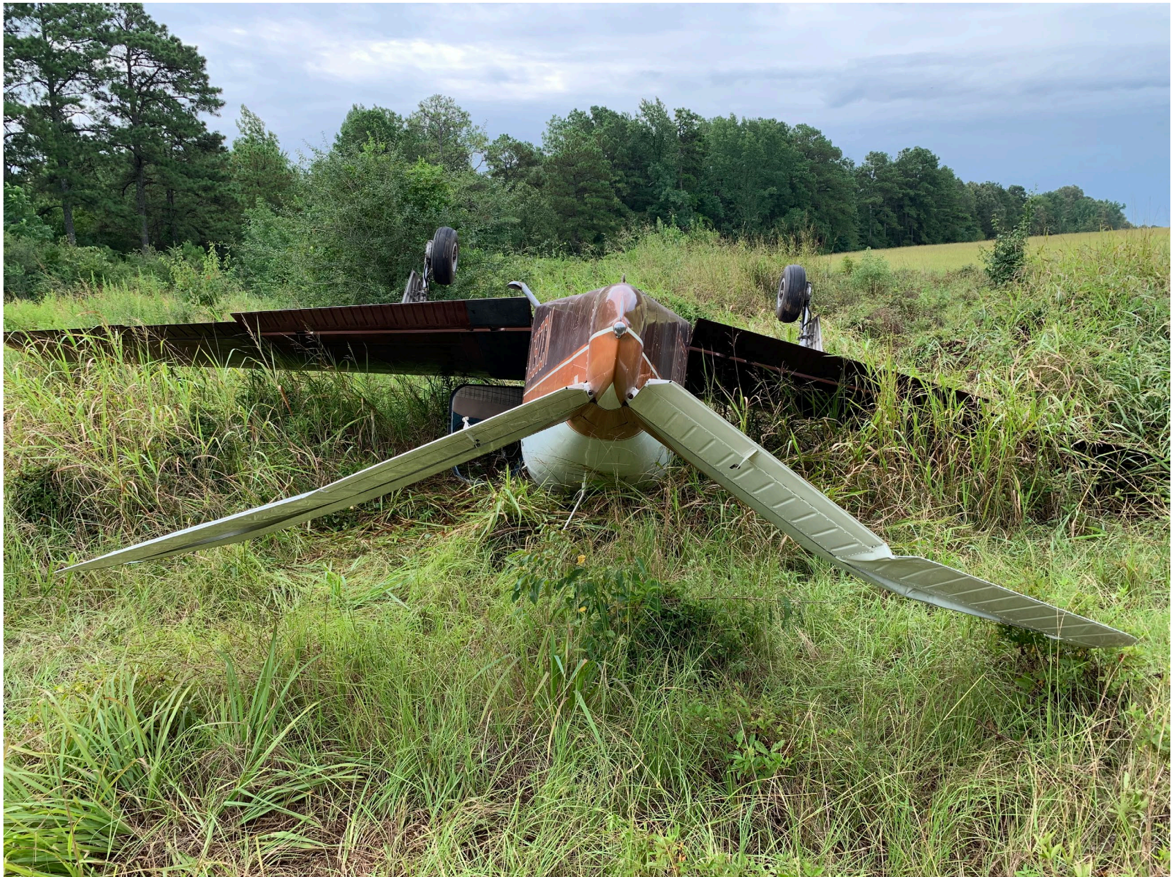
Photo 2 – Damage to ruddervator and stabilizer (Photo courtesy FAA).
