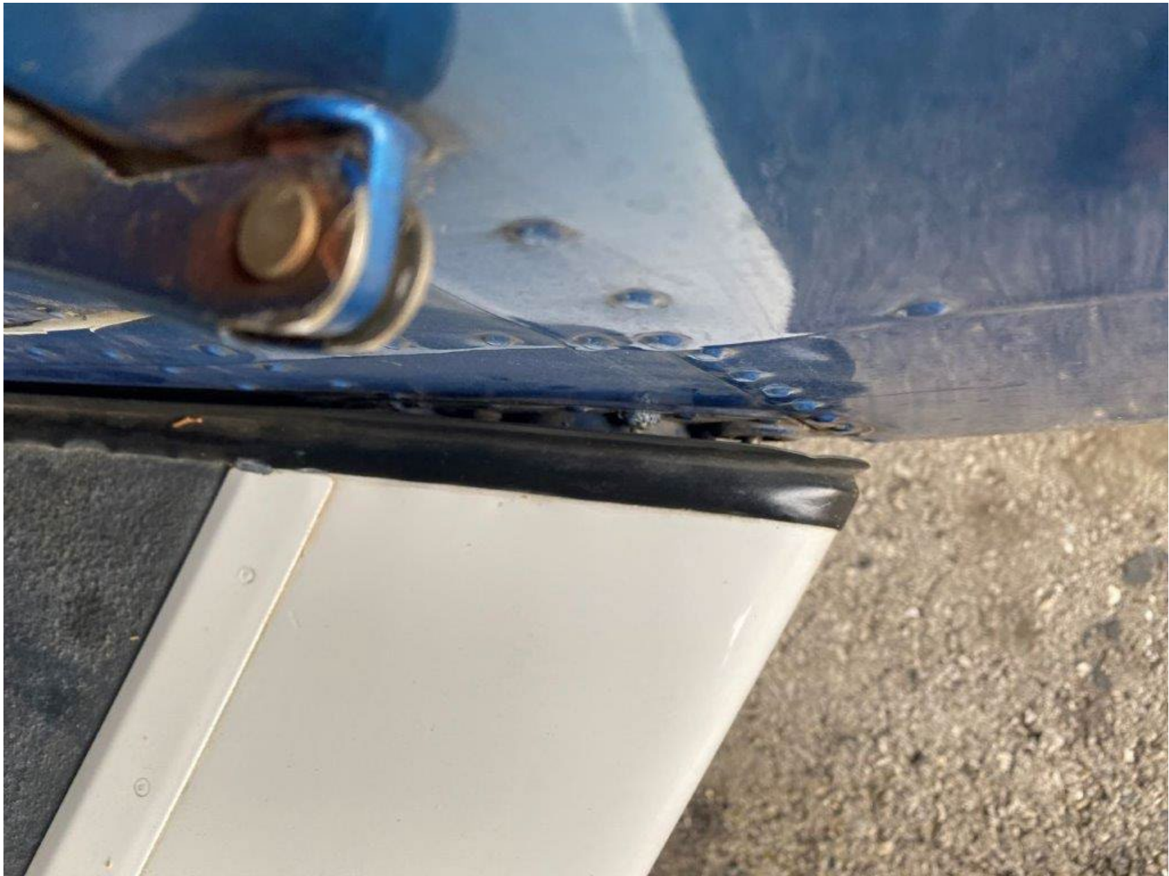
Photo 3 - Ring Wing Damage (Courtesy of KEOS Airport Manager)
