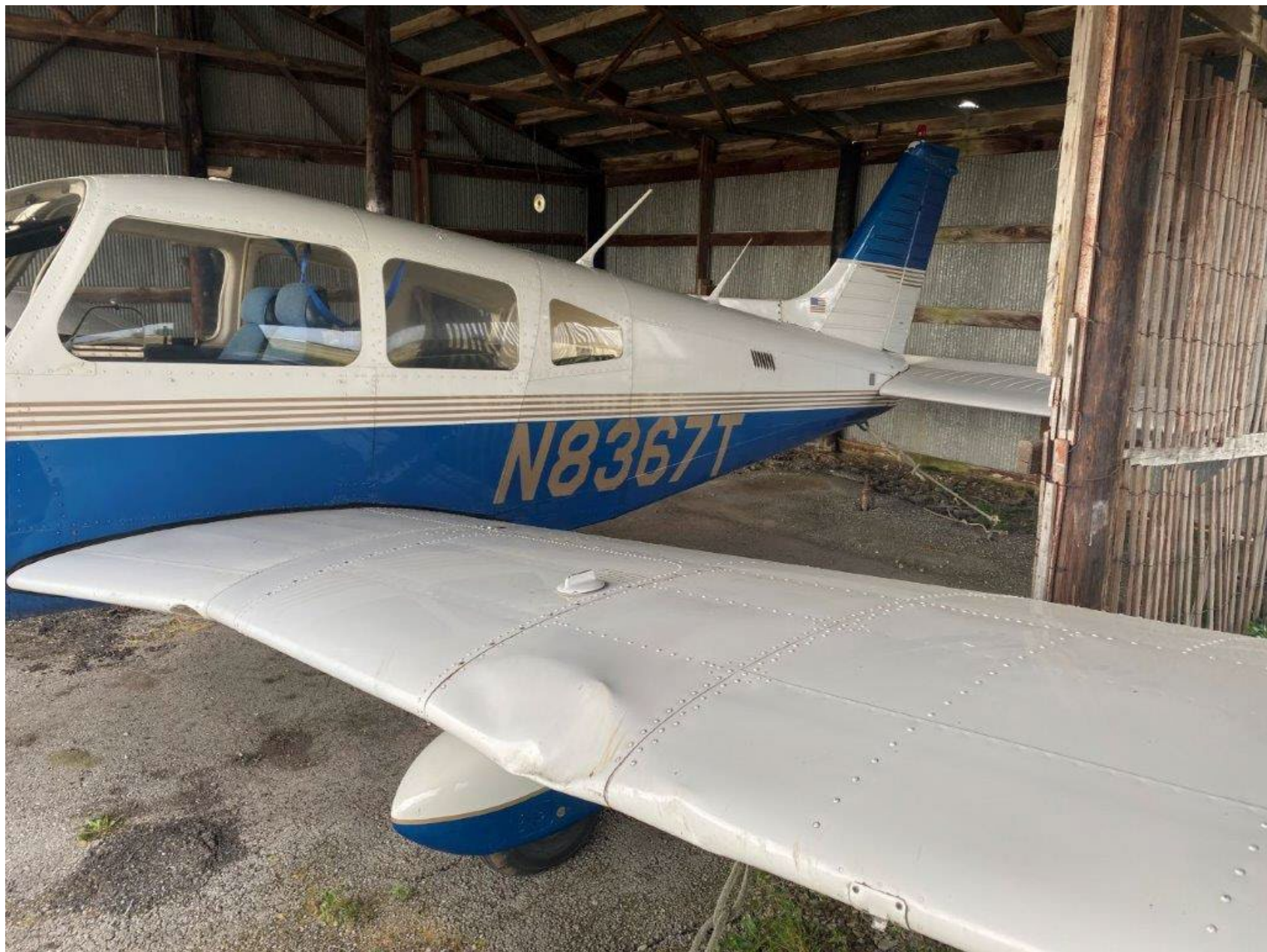
Photo 4 - Left Wing Damage (Courtesy of KEOS Airport Manager)
