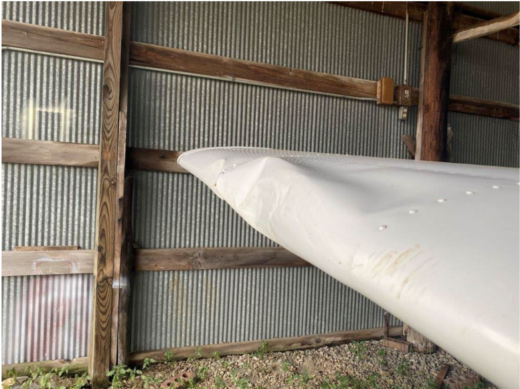
Photo 5 – Ring Wing Damage (Courtesy of KEOS Airport Manager)
