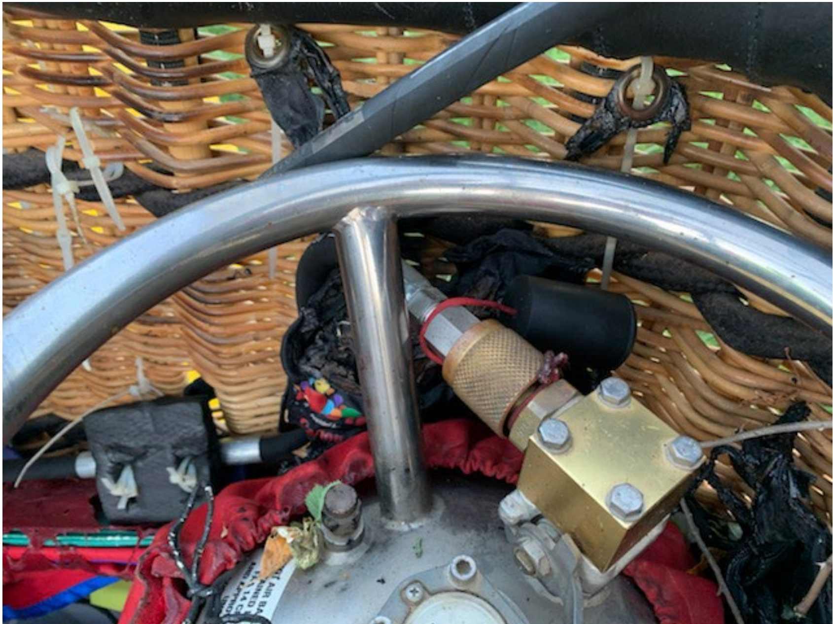
Photo 6 – Close Up of Propane Tank and Fittings (Photo Provide by FAA)
