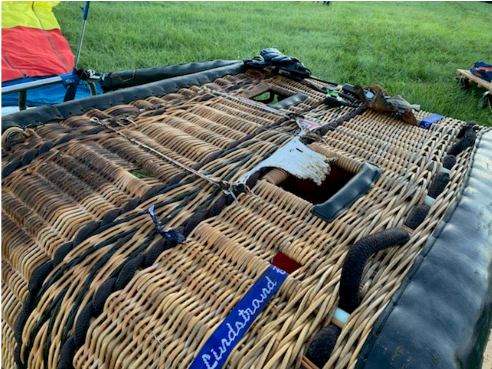
Photo 2 – Basket Side / Burn Marks (Photo Provided by FAA)
