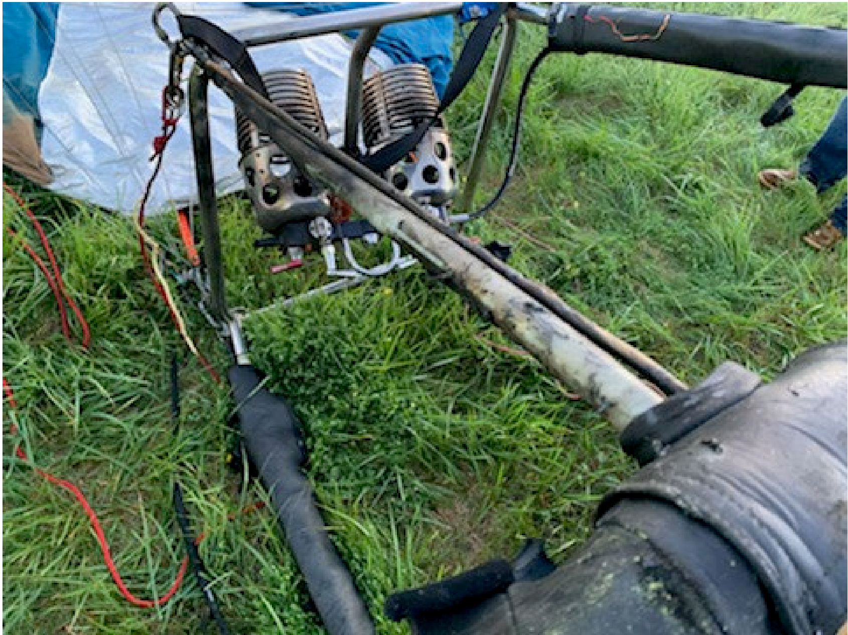
Photo 3 – Burn Indications on Frame / Burners (Photo Provided by FAA)
