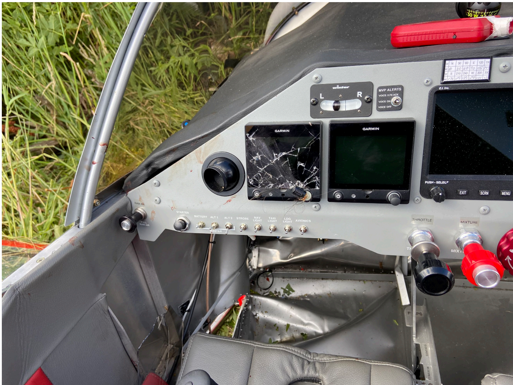
Photo 2 – View of the substantial damage sustained to the fuselage at the accident site (courtesy of the Federal Aviation Administration).
