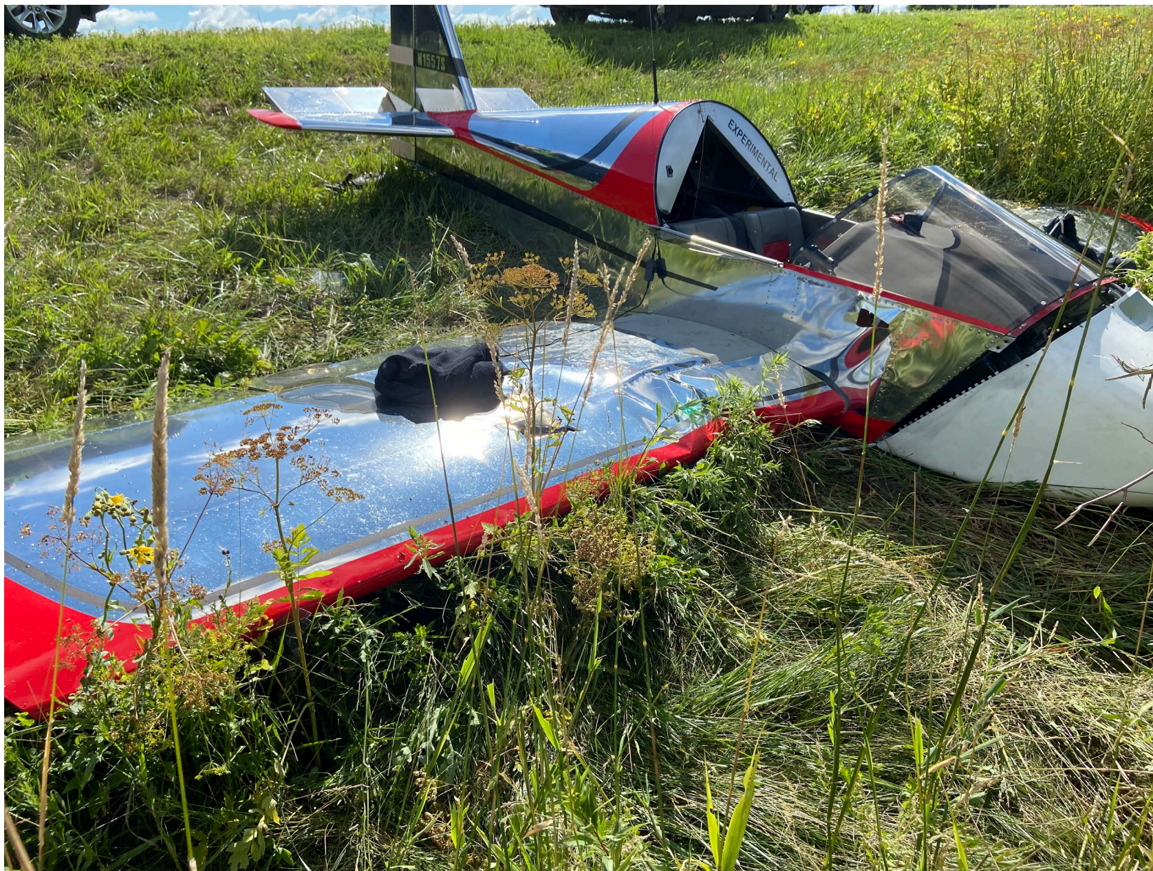
Photo 1 – View of the substantial damage sustained to the right wing at the accident site (courtesy of the Federal Aviation Administration).
