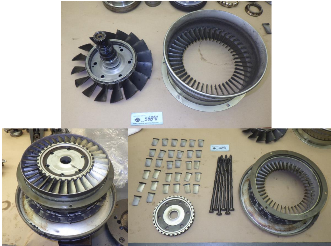
Photo No. 21 1 st , 2 nd & 3 rd stage compressor rotors
