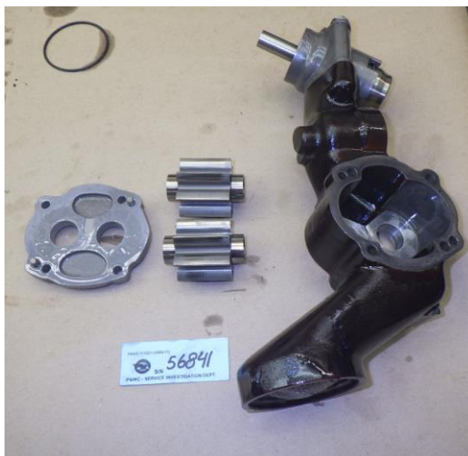
Photo No. 28 Oil Pressure Pump
