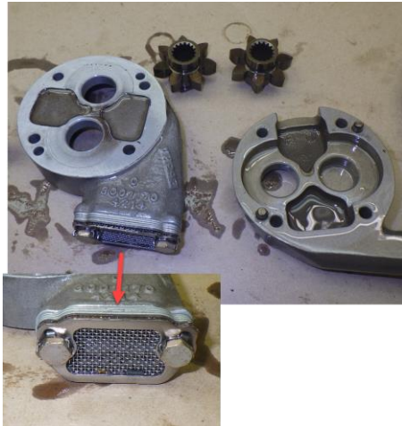
Photo No. 30 No. 2 bearing oil scavenge pump
