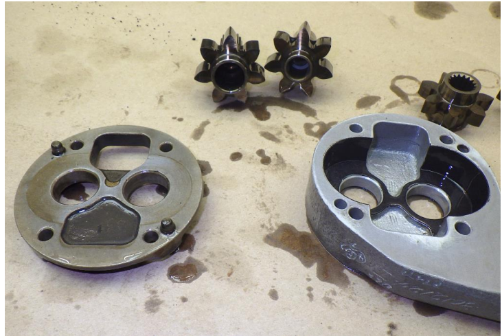
Photo No. 31 AGB oil scavenge pump
