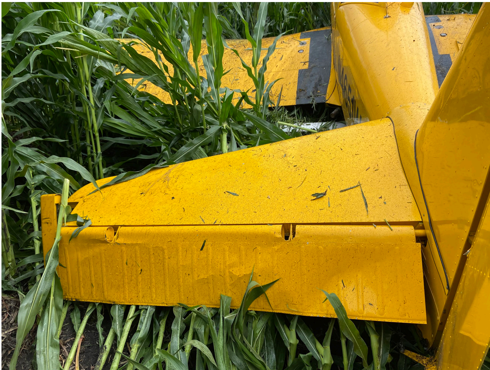
Photo 2 – Horizontal Stabilizer (Provided by FAA)
