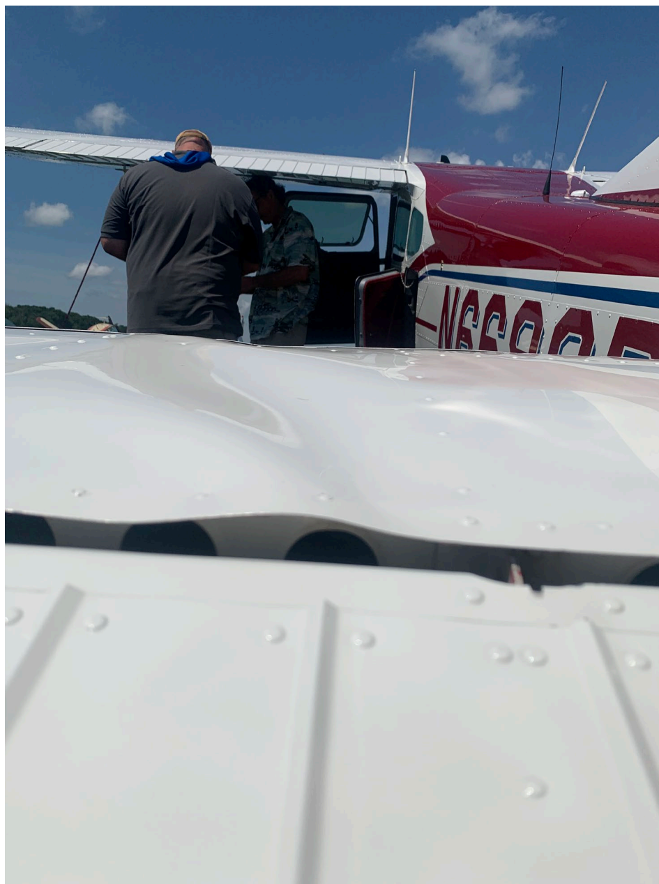
Photo 2 – Left horizontal stabilizer (Provided by FAA)
