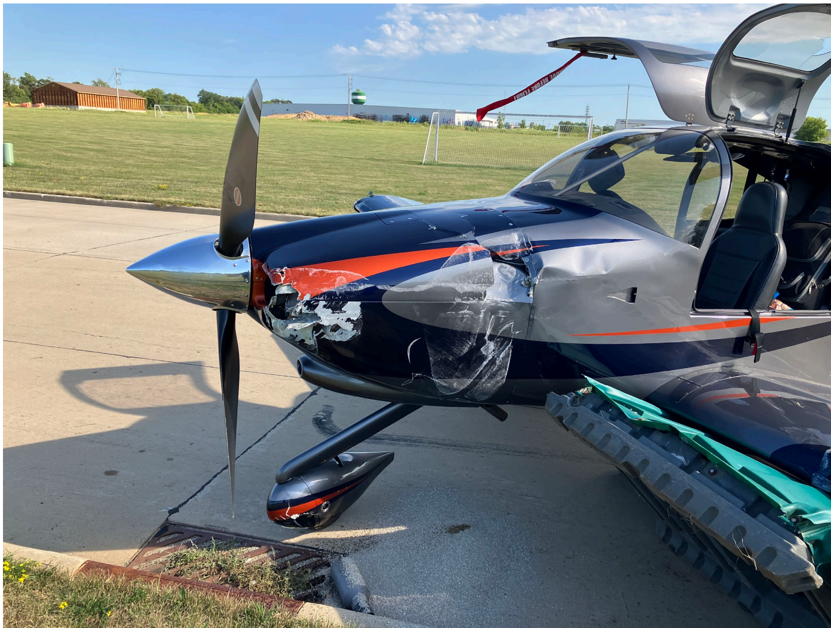
Photo 5 – View of the propeller and the engine at the accident site (courtesy of the Federal Aviation Administration).
