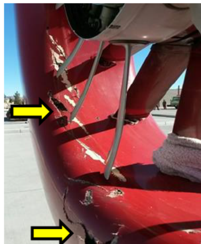
Figure 2. Lower fenestron housing.
