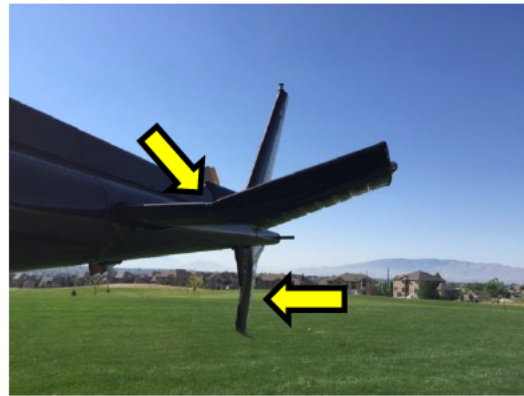
Figure 4. Empennage (horizontal stabilizer and vertical fin).
