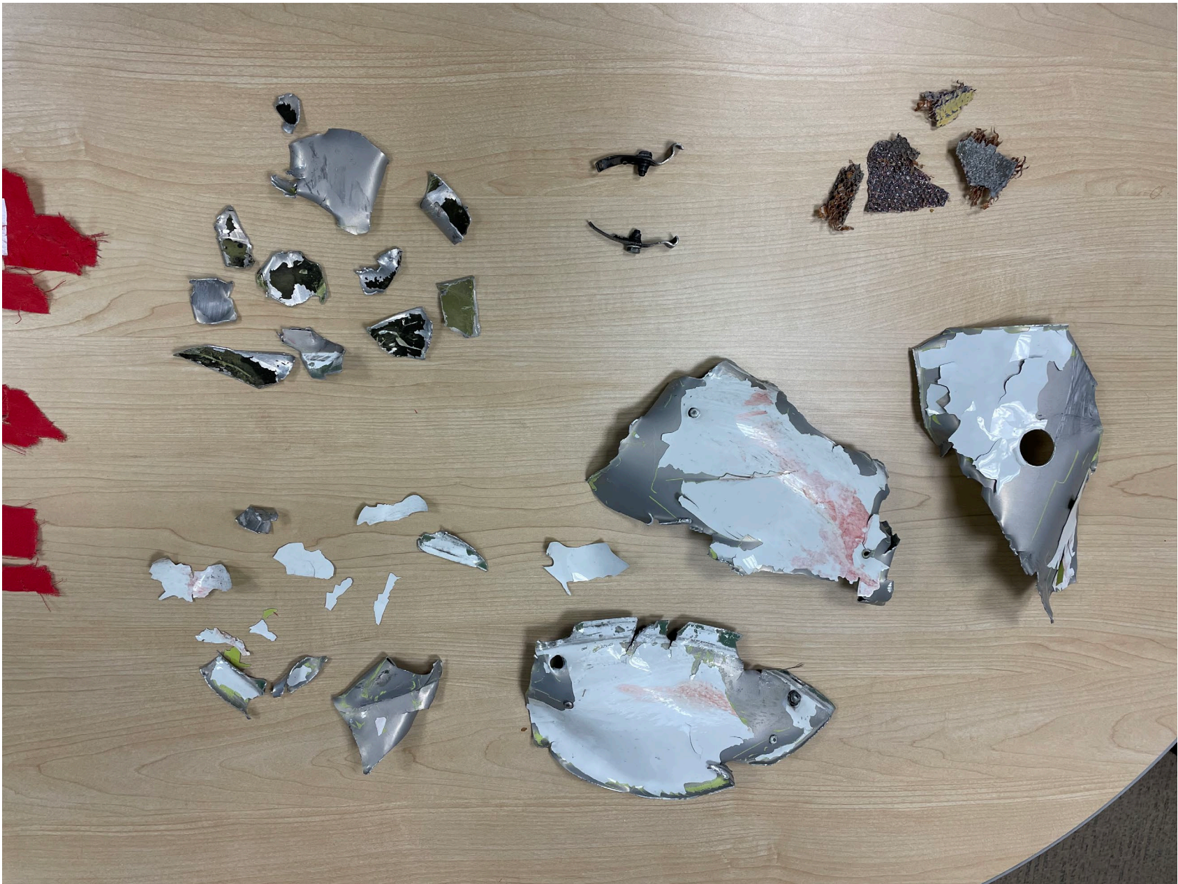
Photo 6 – View of the metal fenestron hub cover (courtesy of the operator).
