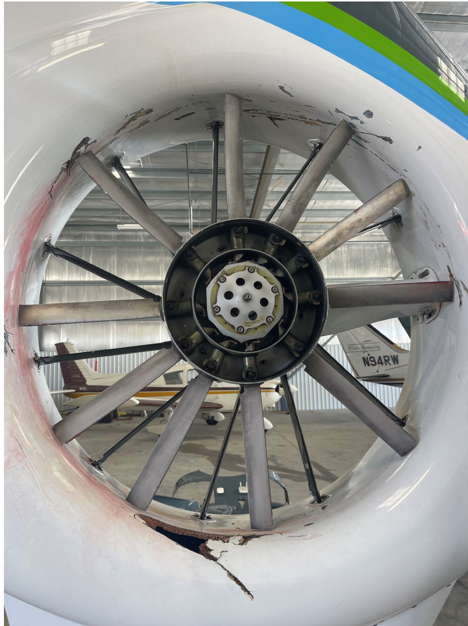
Photo 1 – View of the right side of the fenestron assembly (courtesy of the operator).
