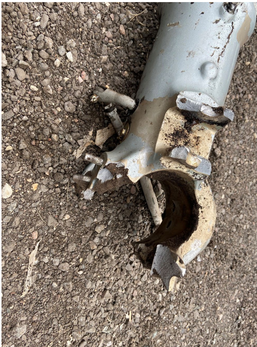
Photograph 4 - Main Rotor Mast Hub (Courtesy of FAA)
