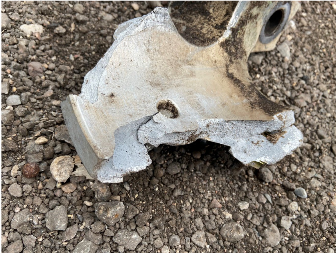
Photograph 3 - Fractured Rotor Hub (Courtesy of FAA)
