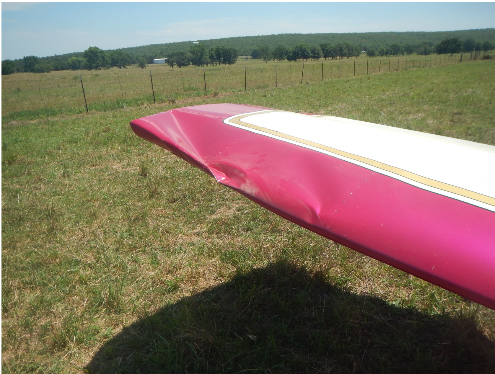
Photo 4 – Right Wing Damage (photograph provided by airplane owner)
