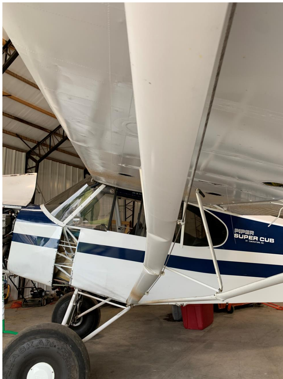
Photo 2 – Accident Airplane / Left Wing Strut (Provide by FAA)
