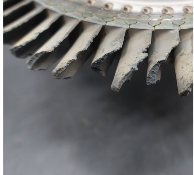
Photo 12- CT Rotor Blades, Trailing Edge, (R) CT Blade Fracture Surfaces
