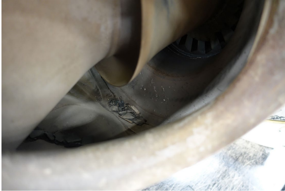
Photo 7- Metal Fragments Collected in Exhaust Duct
