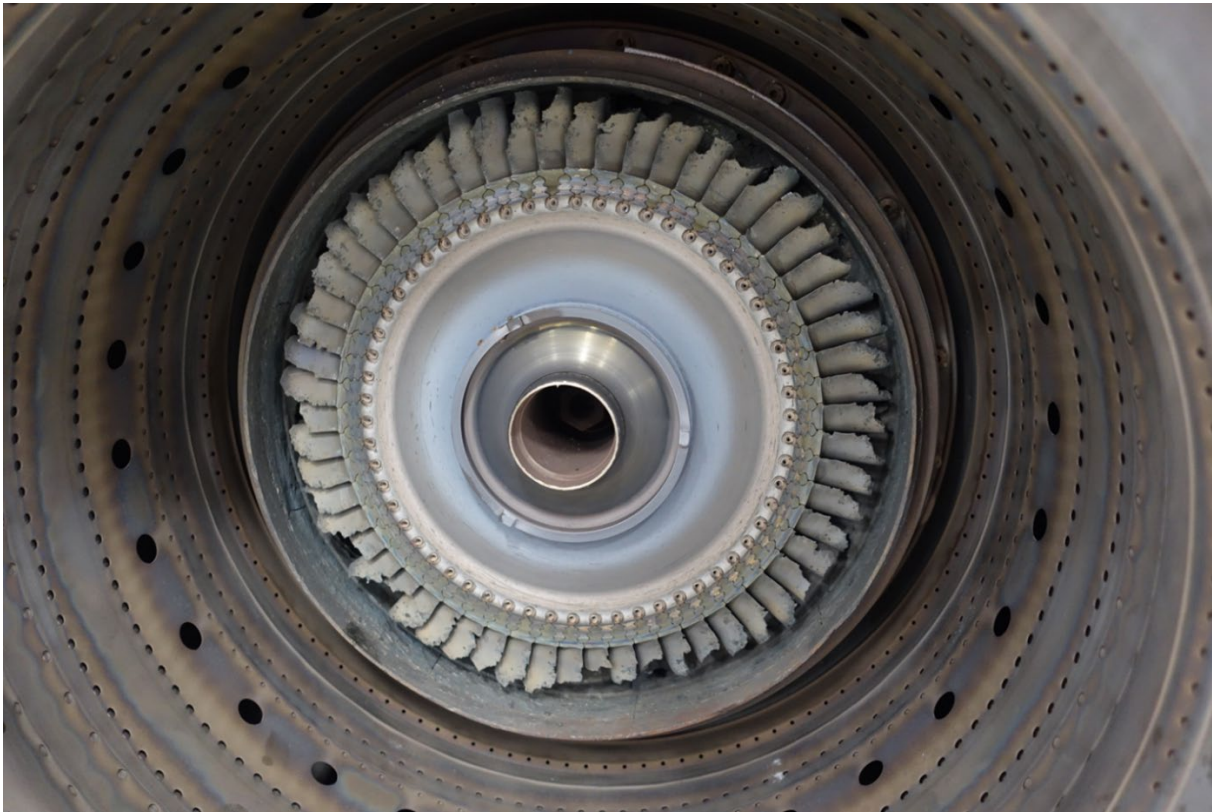
Photo 11- CT Rotor, Trailing Edge, and Combustion Liner
