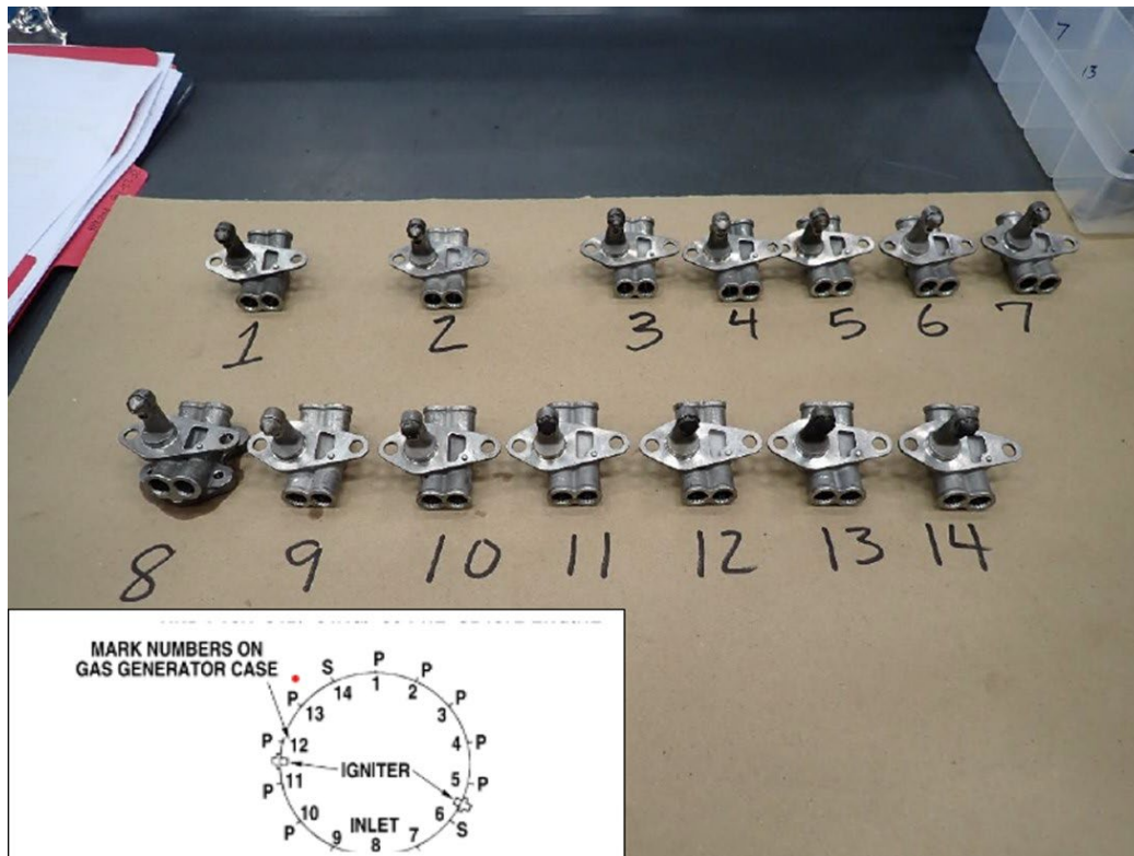
Photo 18- Fuel Nozzle Set, Nozzle Position Identification Diagram (Photo Courtesy of PWC)
