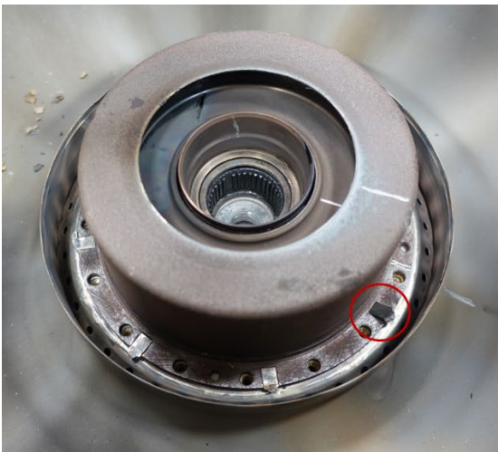
Photo 14- (L) No. 2 Bearing Cover CT Vane Lug Fractures, (R) Impact Marks
