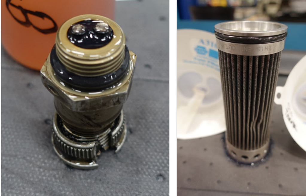
Photo 8- (L) Magnetic Chip Detector, (R) Oil Filter
