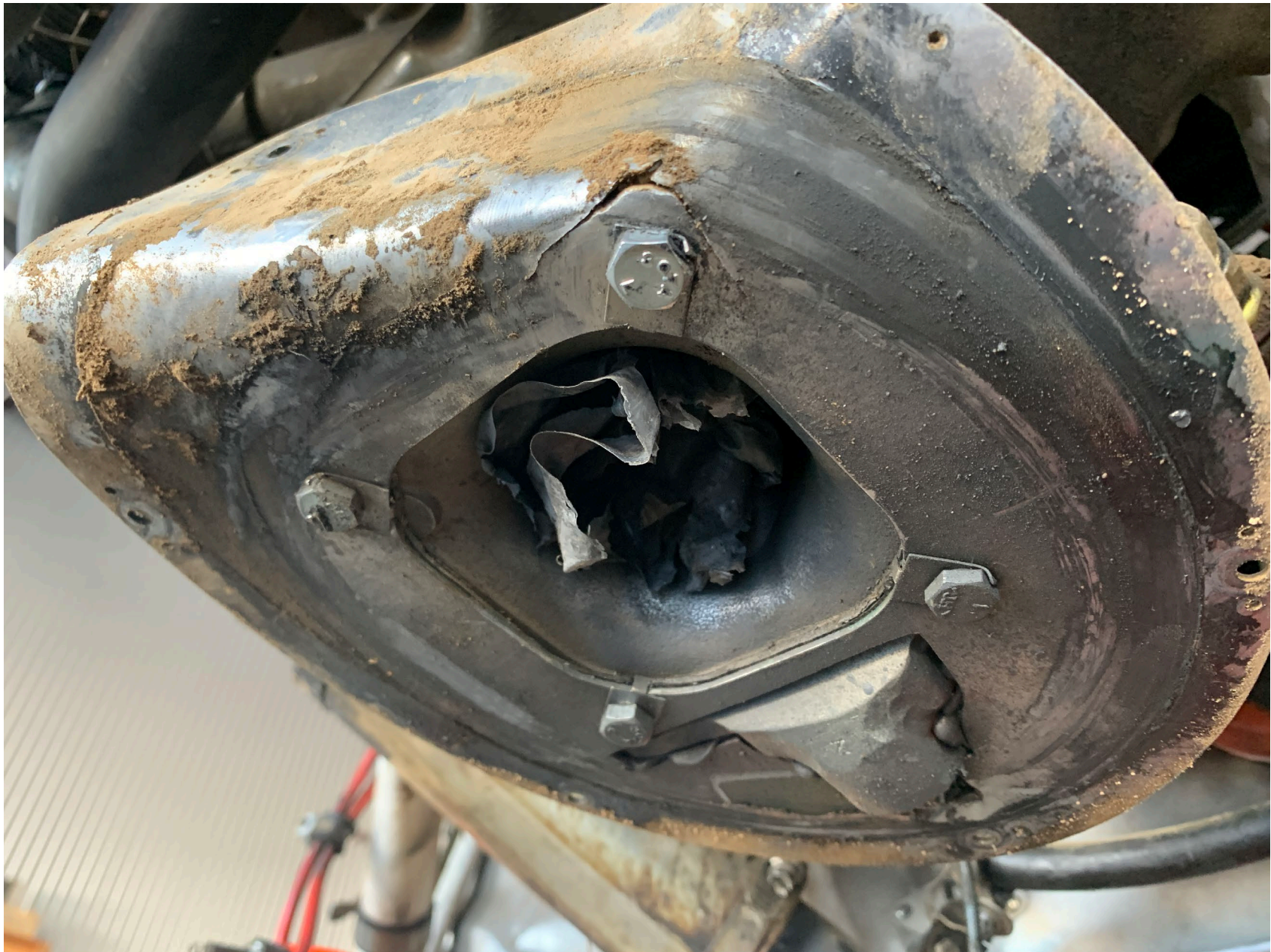
Photo 8 – View of the throttle body with the air box removed, showing foreign object debris lodged in the throttle body.
