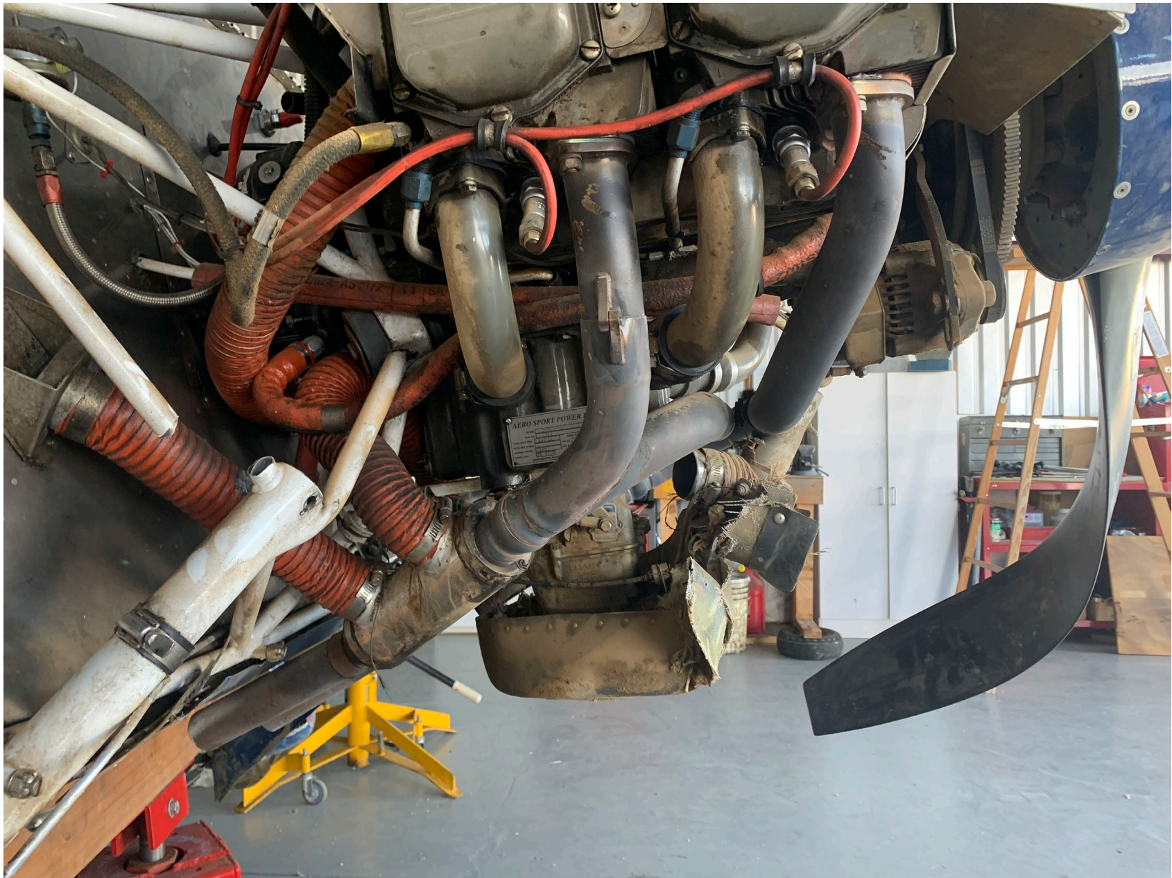
Photo 4 – View of the substantial damage sustained to the right side engine mount.
