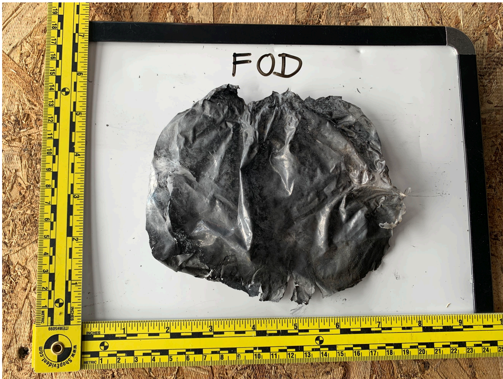
Photo 10 – View of the foreign object debris removed from the throttle body.
