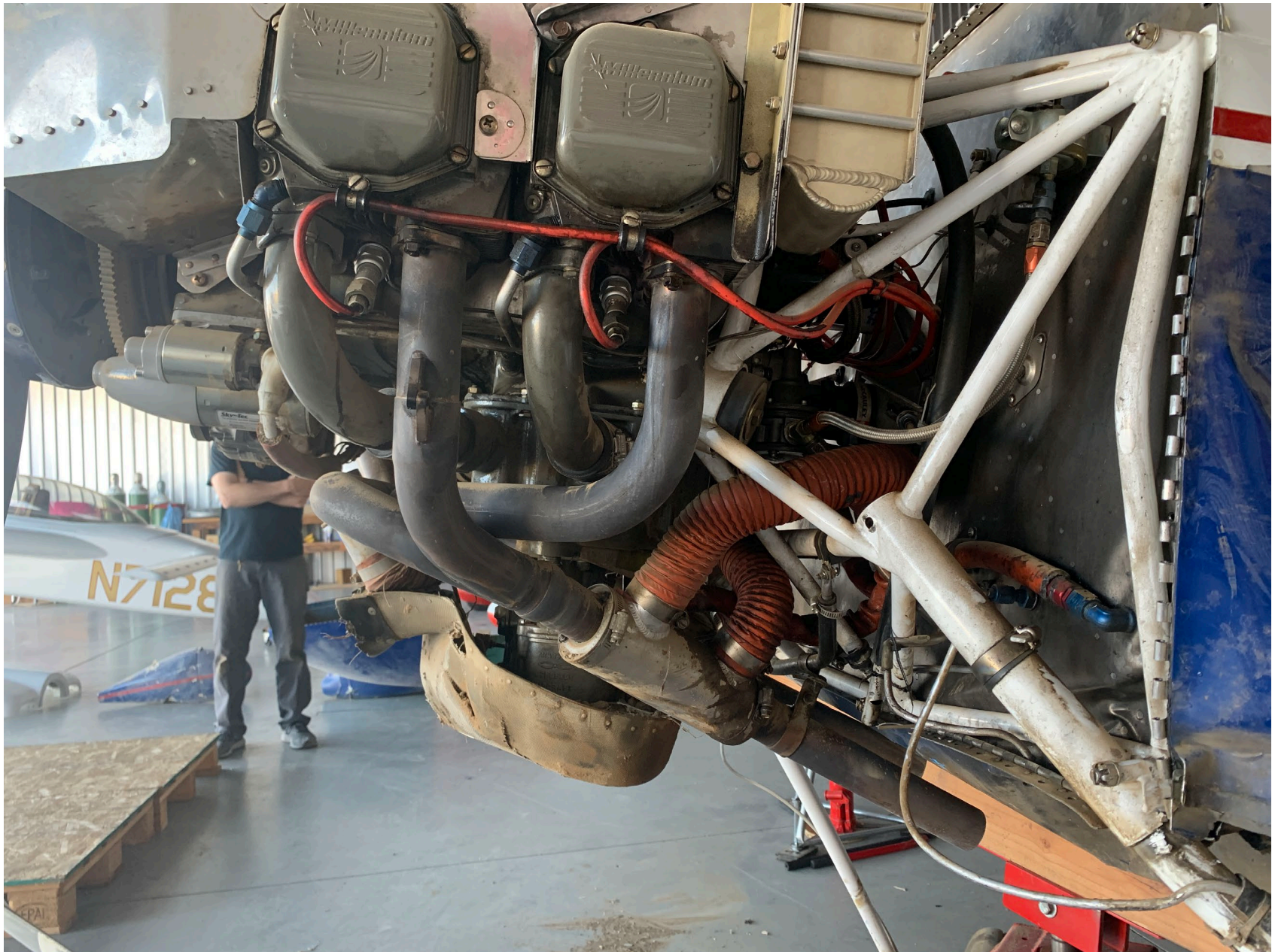
Photo 6 – View of the substantial damage sustained to the left side engine mount.
