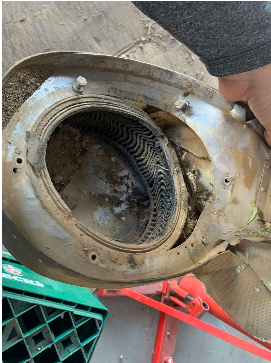
Photo 7 – View of the air box removed from the engine.
