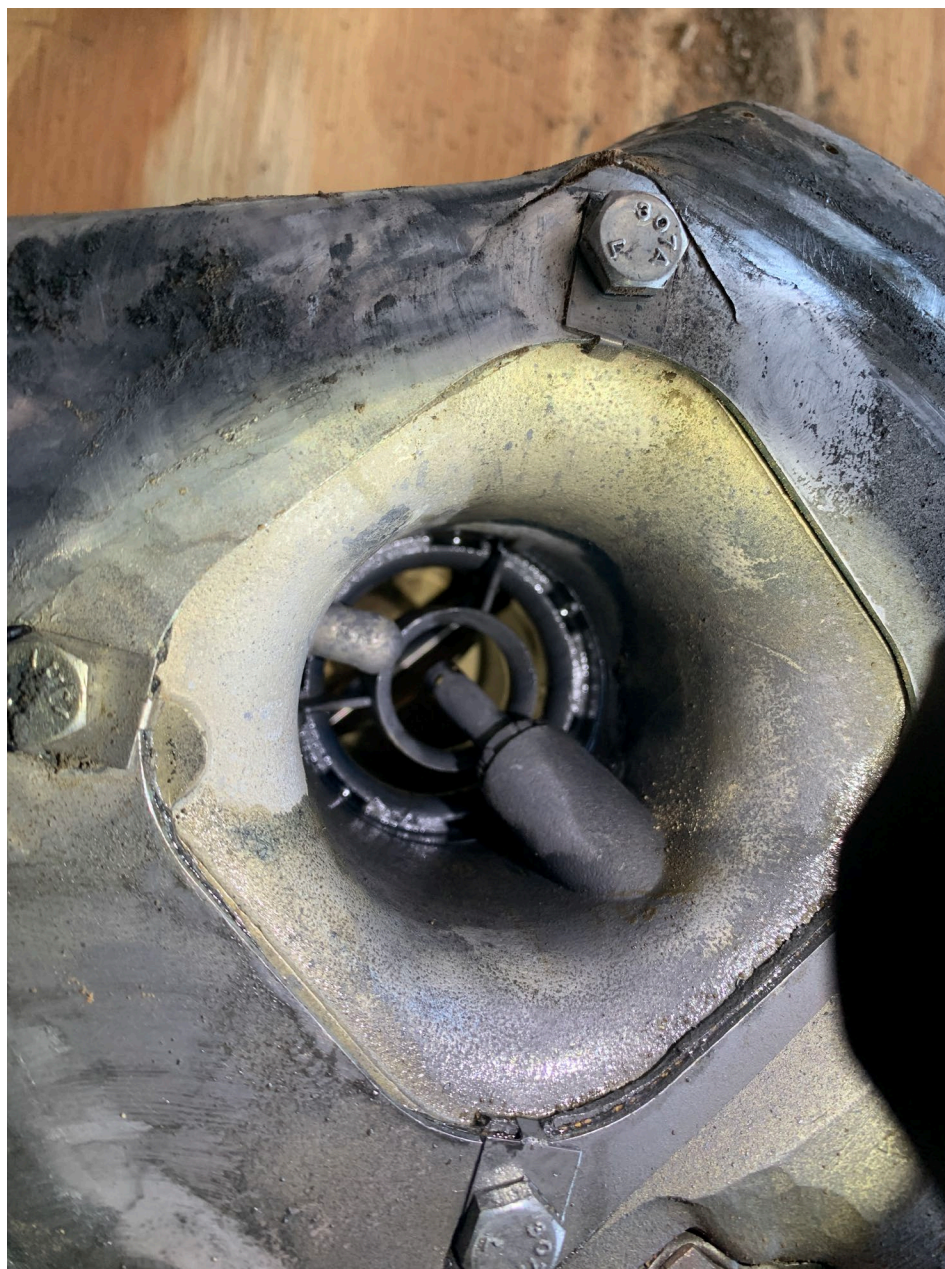
Photo 9 – View of the throttle body once the foreign object debris was removed.
