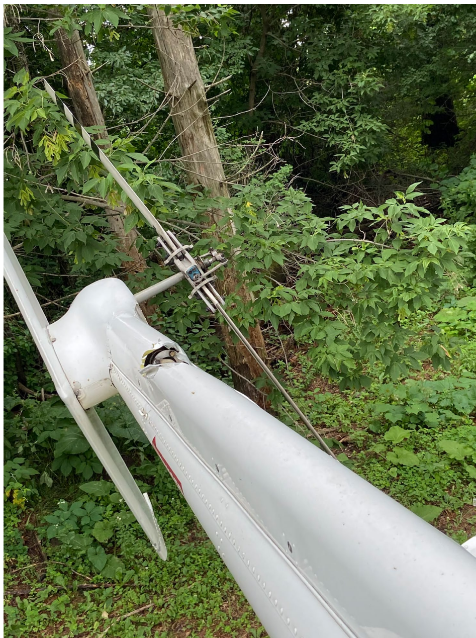
Photo 3 – Damage to tail boom (Photo courtesy of FAA)
