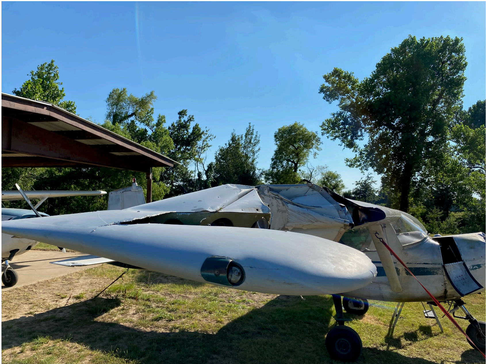
Photo 2 – Right Wing Damage – Photo Courtesy of FAA
