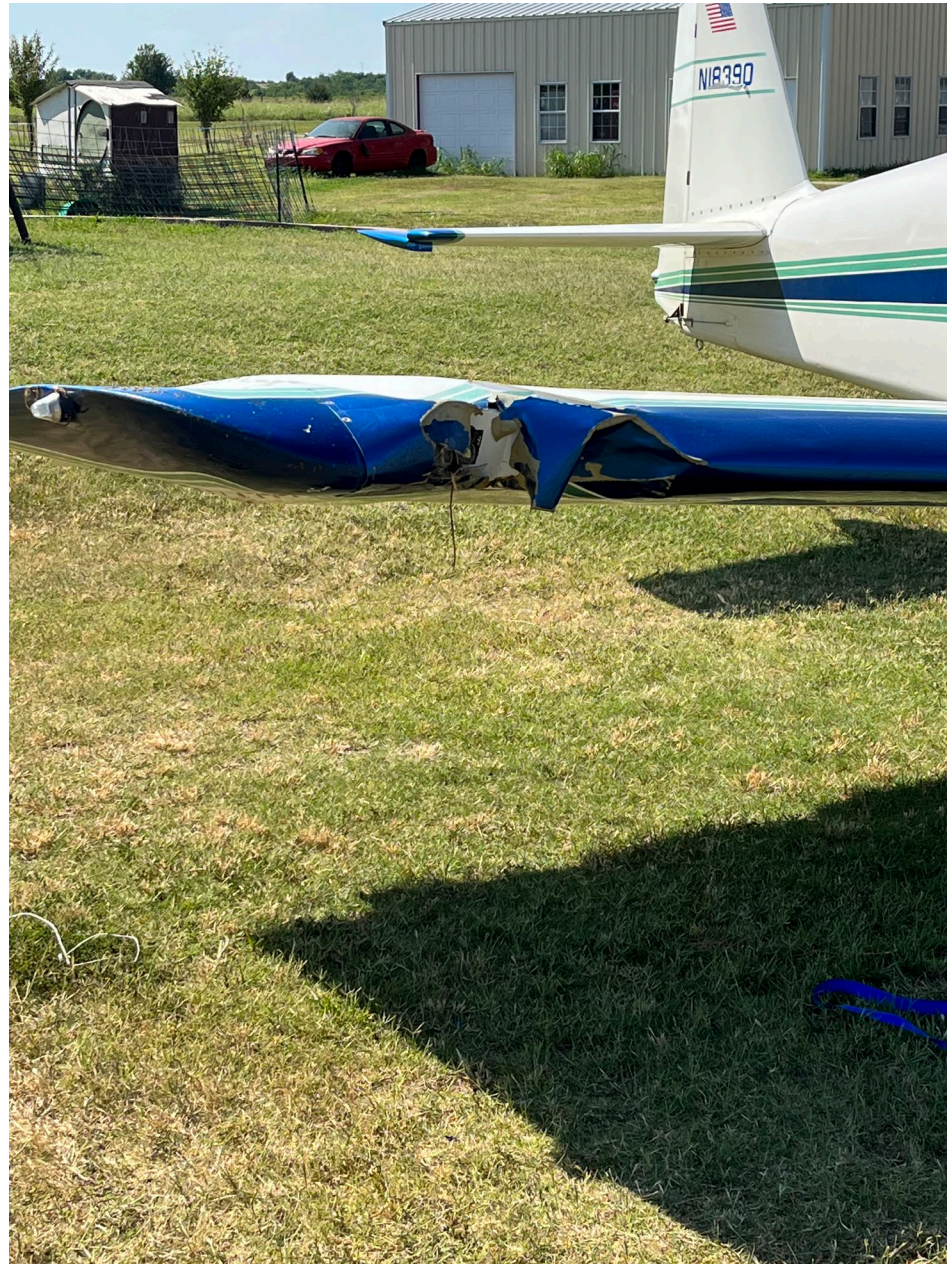
Photo 2 – Right Wing Leading Edge Damage – Courtesy of FAA
