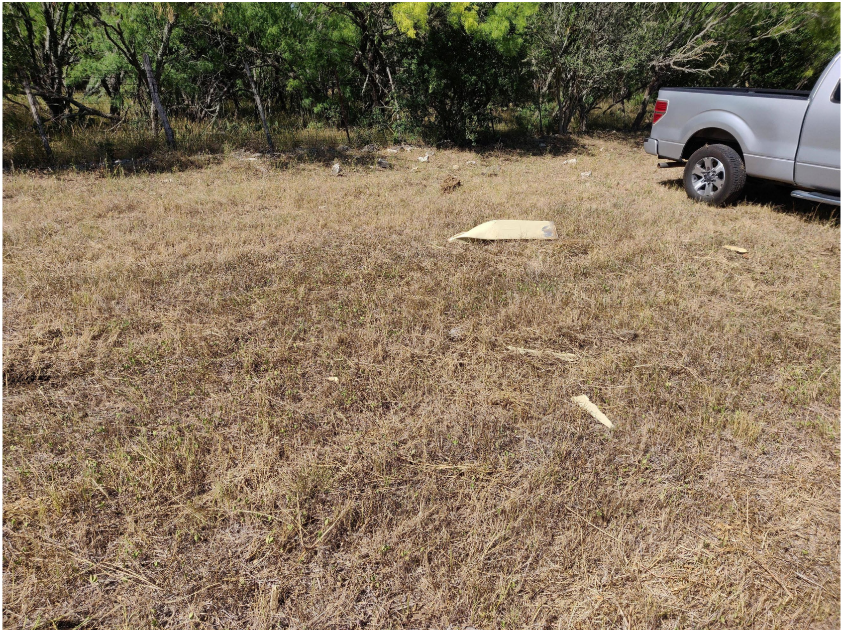
Photo 3 – Ring wing sponson separated from airplane (Photo provided by pilot)
