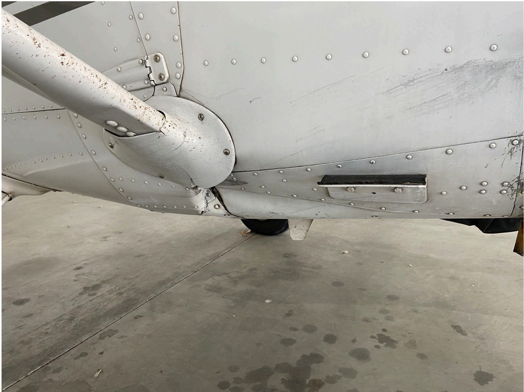
Photo 1 – Damage to fuselage near right wing strut (FAA photo)
