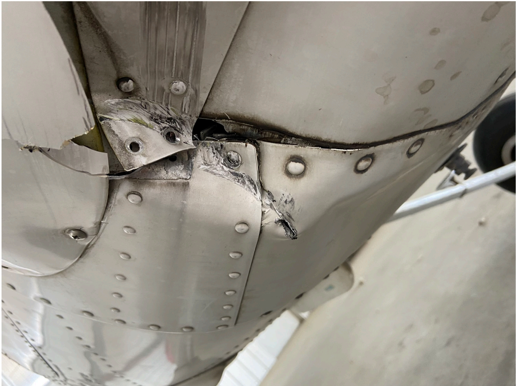
Photo 2 – Additional photo of damage near right wing strut (FAA photo)
