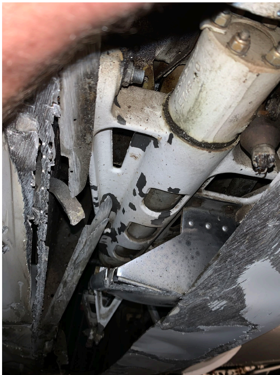
Photo 4 – View of the underside of the fuselage, showing the substantial damage (courtesy of the Federal Aviation Administration).
