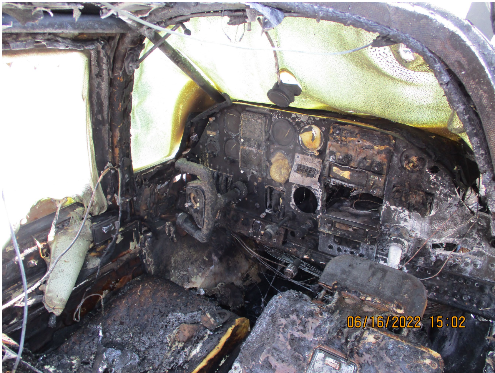
Photo 2 – Fire Damaged Cockpit, Courtesy of FAA
