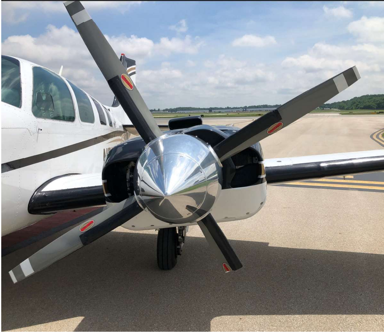
Photo #1 – Left propeller with one blade fractured
