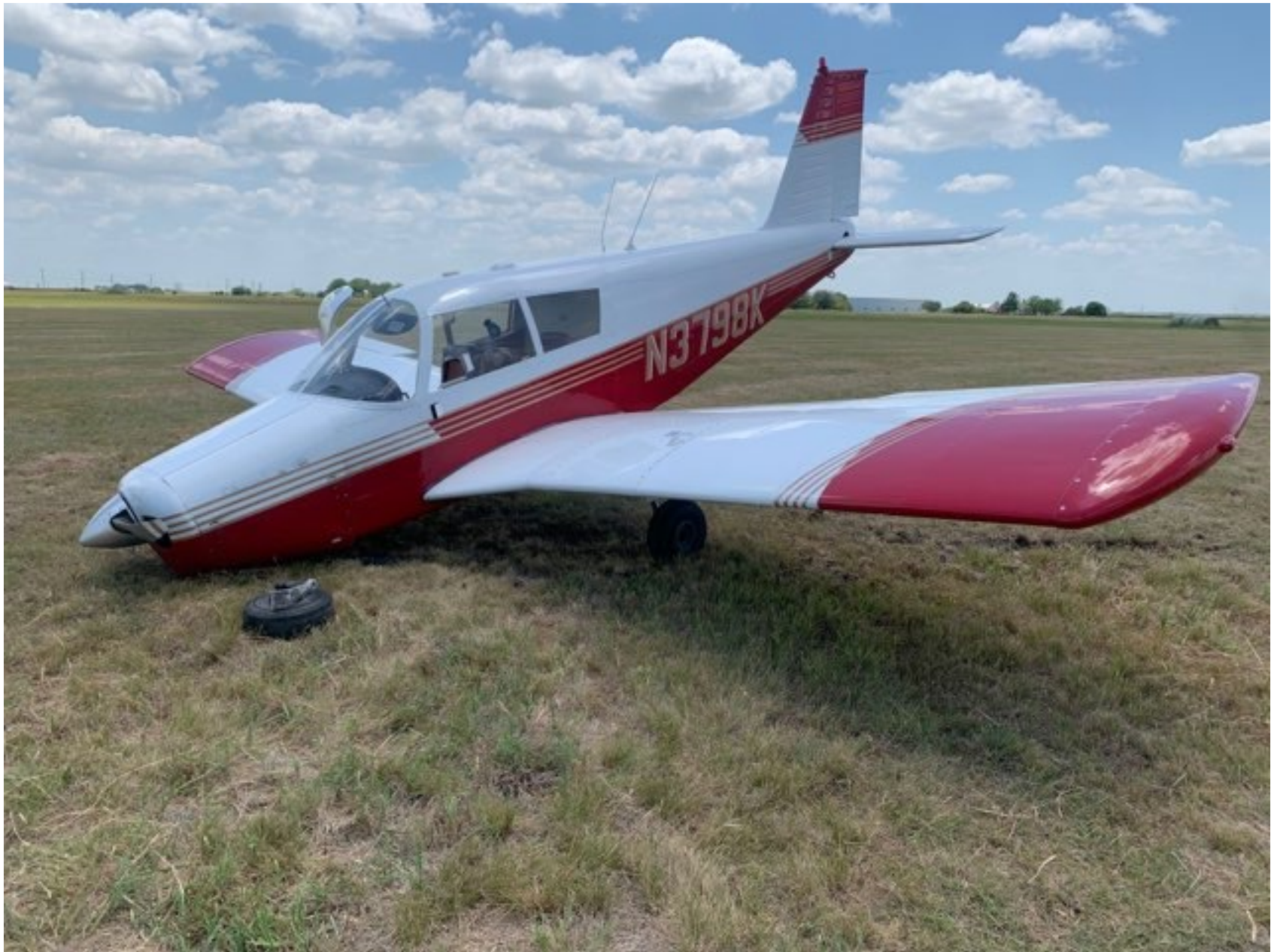
Photo 1 – Collapsed nose wheel – Courtesy of FAA – (Federal Aviation Administration)
