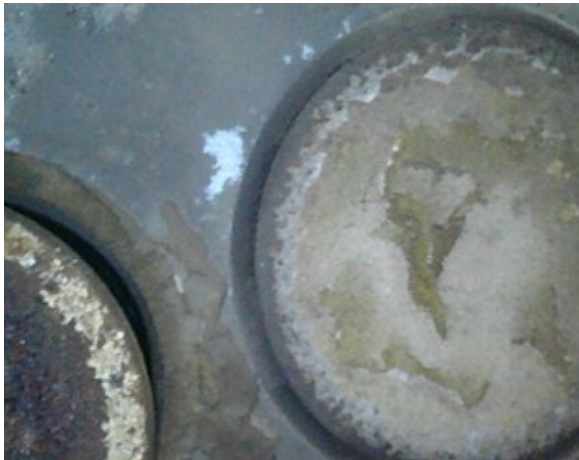
Photo 3 Recessed Intake Valve (Courtesy of Lycoming)
