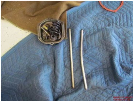
Photo 1 Bent Push Rod (Courtesy of Lycoming)
