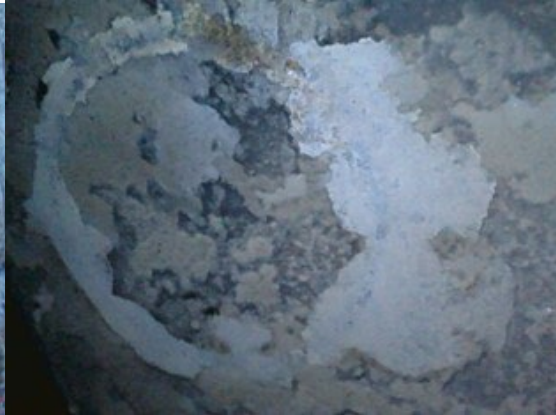
Photo 2 Valve Impression on Top of Piston (Courtesy of Lycoming)
