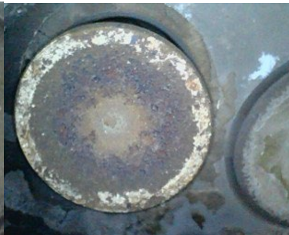
Photo 4 Impact Marks on Exhaust Valve (Courtesy of Lycoming)
