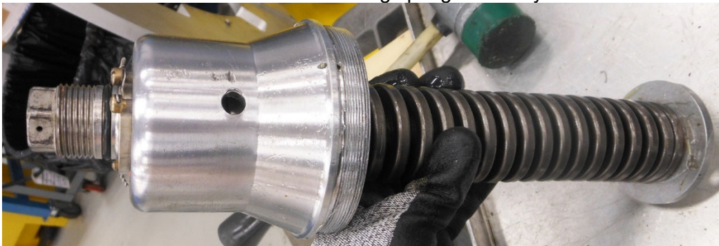
Photo #14 - Feathering spring assembly
