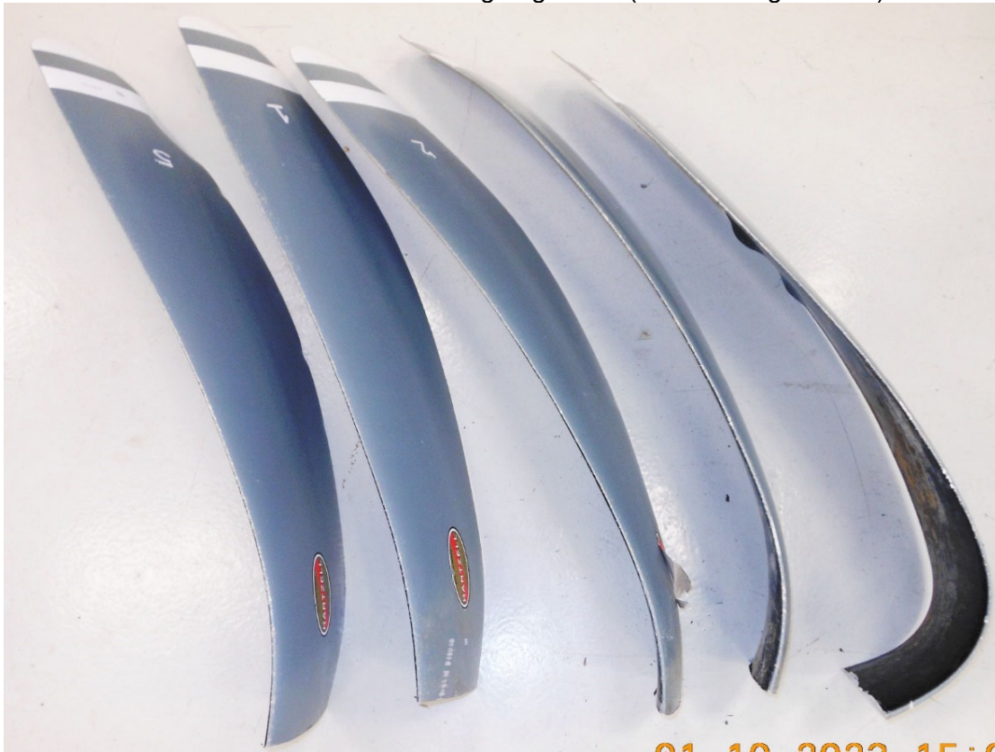
Photo #21 – Blade bend leading edge view (4-3-2-1-5 right to left)
