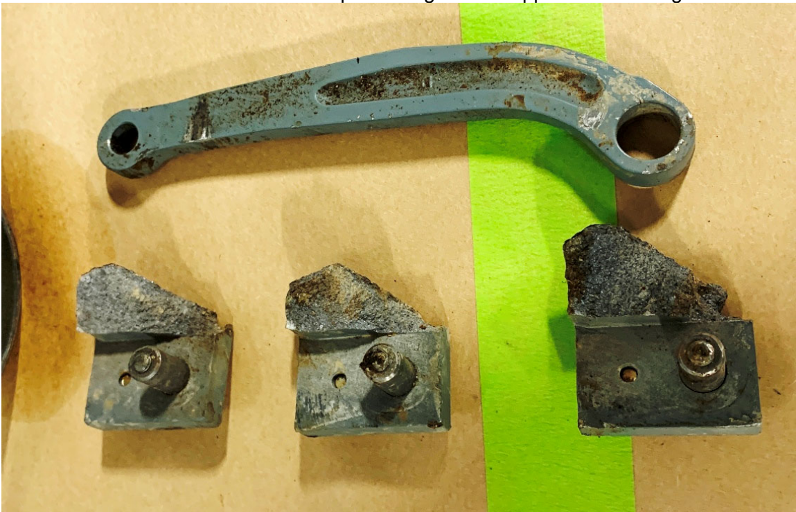
Photo #6 - Link arm and piston fragments shipped loose in bag
