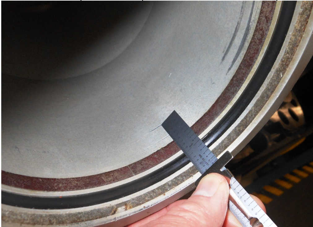
Photo #11 – Representative impact marks on internal surface of piston
