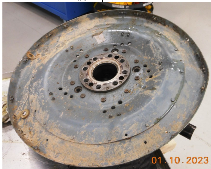
Photo #8 - Spinner bulkhead
