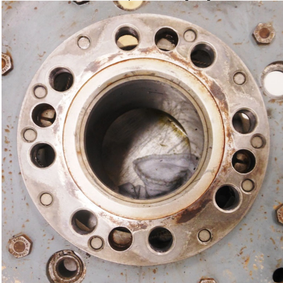
Photo #9 - Propeller mounting flange
