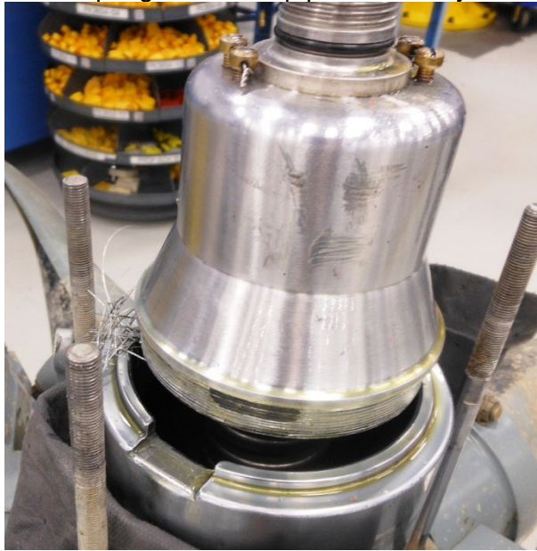
Photo #13 - Spring retainer cup pulled from cylinder mount
