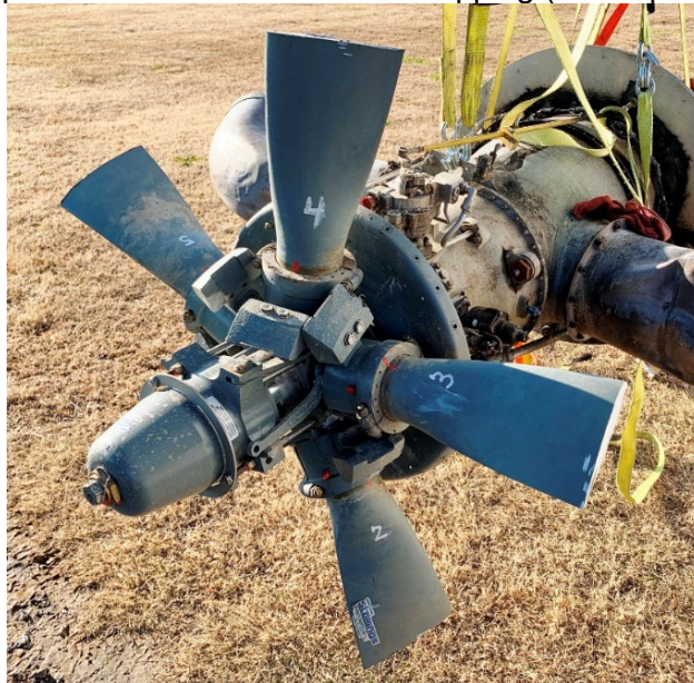
Photo #3 – Propeller blades cut to facilitate shipping (Photo provided by NTSB)
