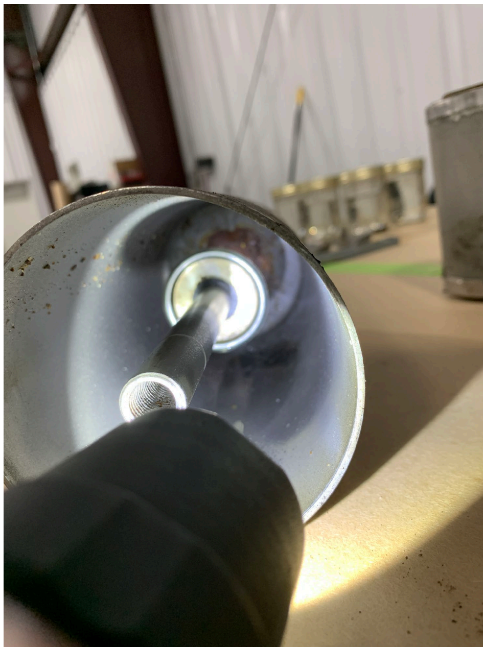
Photo 20 – View of the inside of the firewall fuel filter bowl, with contamination.
