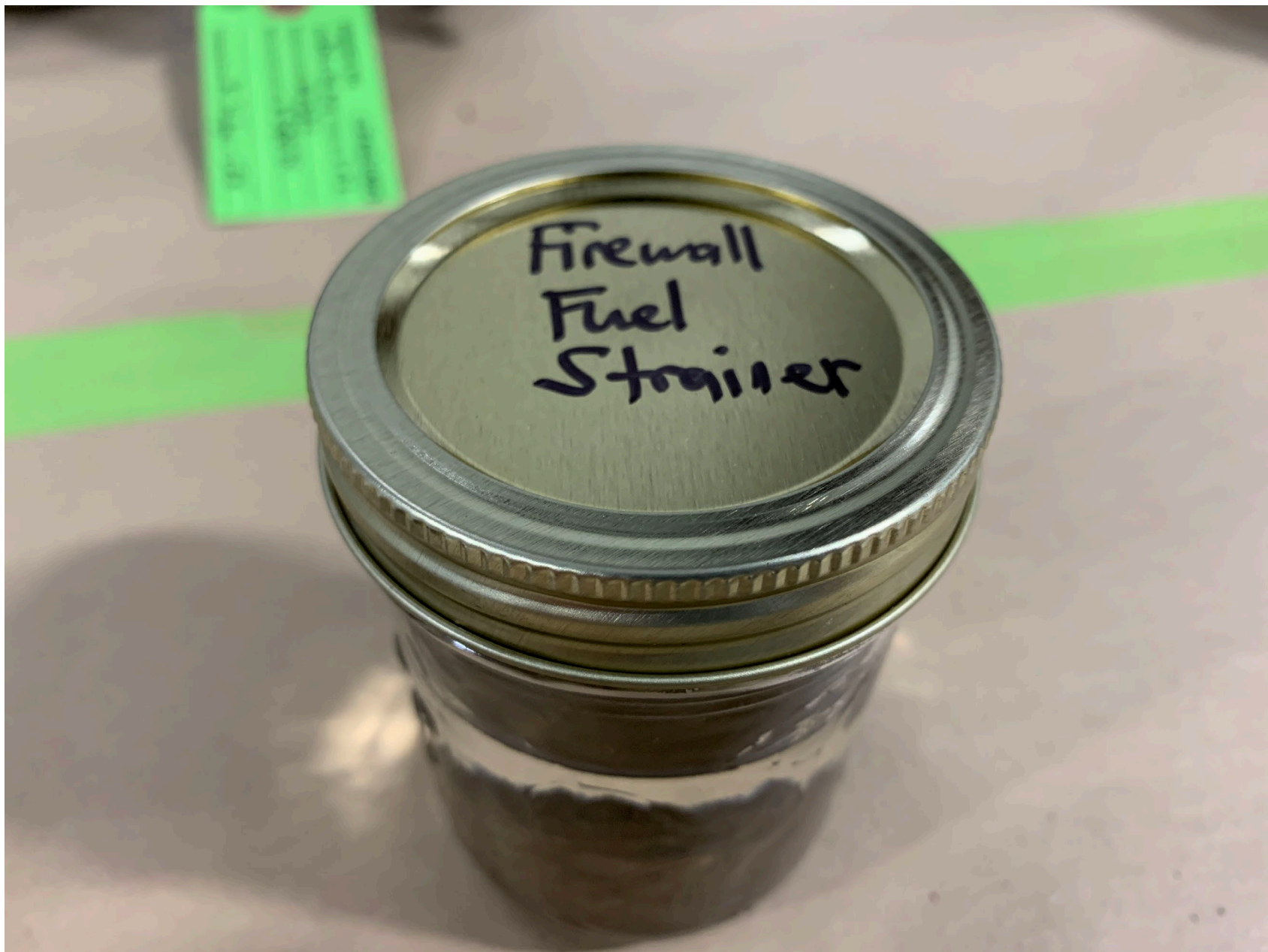
Photo 14 – View of the fuel sample, with contamination, obtained from the firewall fuel filter bowl.
