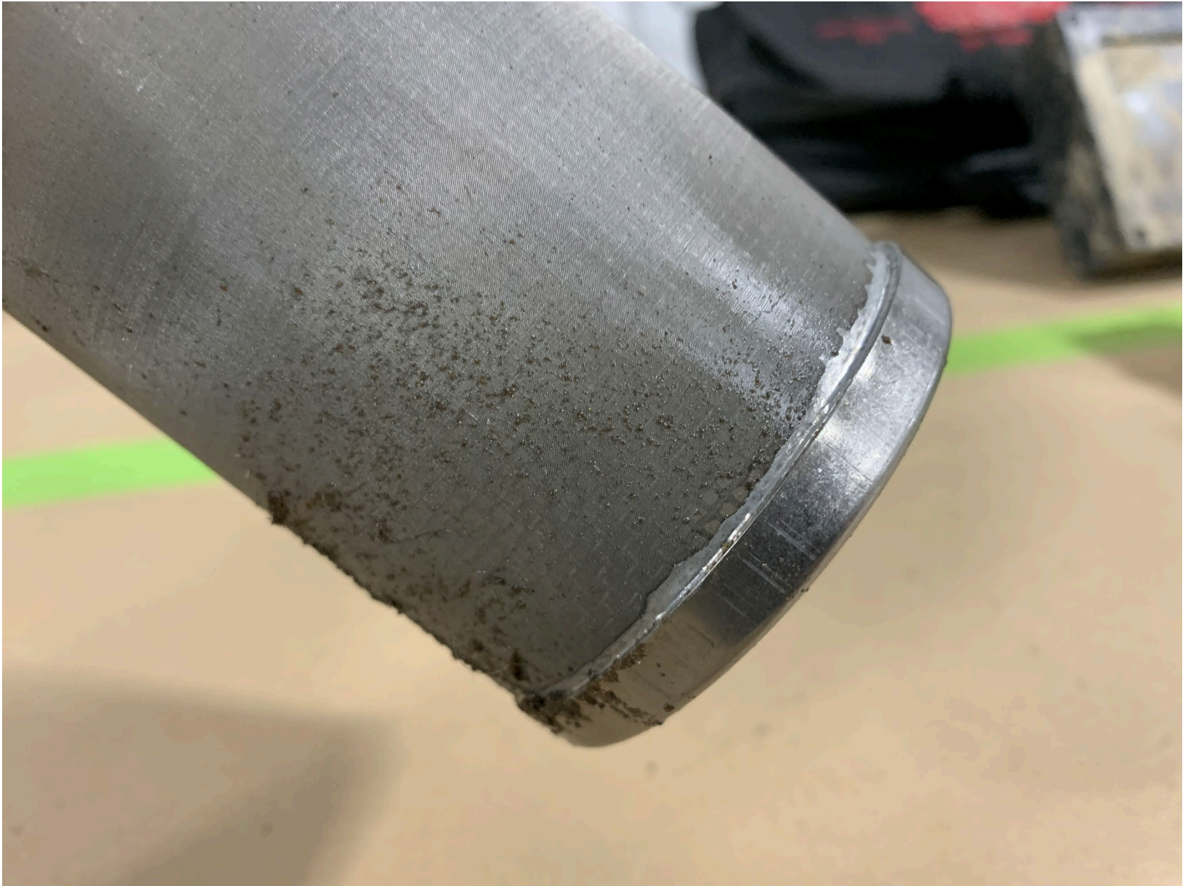
Photo 19 – View of the firewall fuel filter, with contamination.
