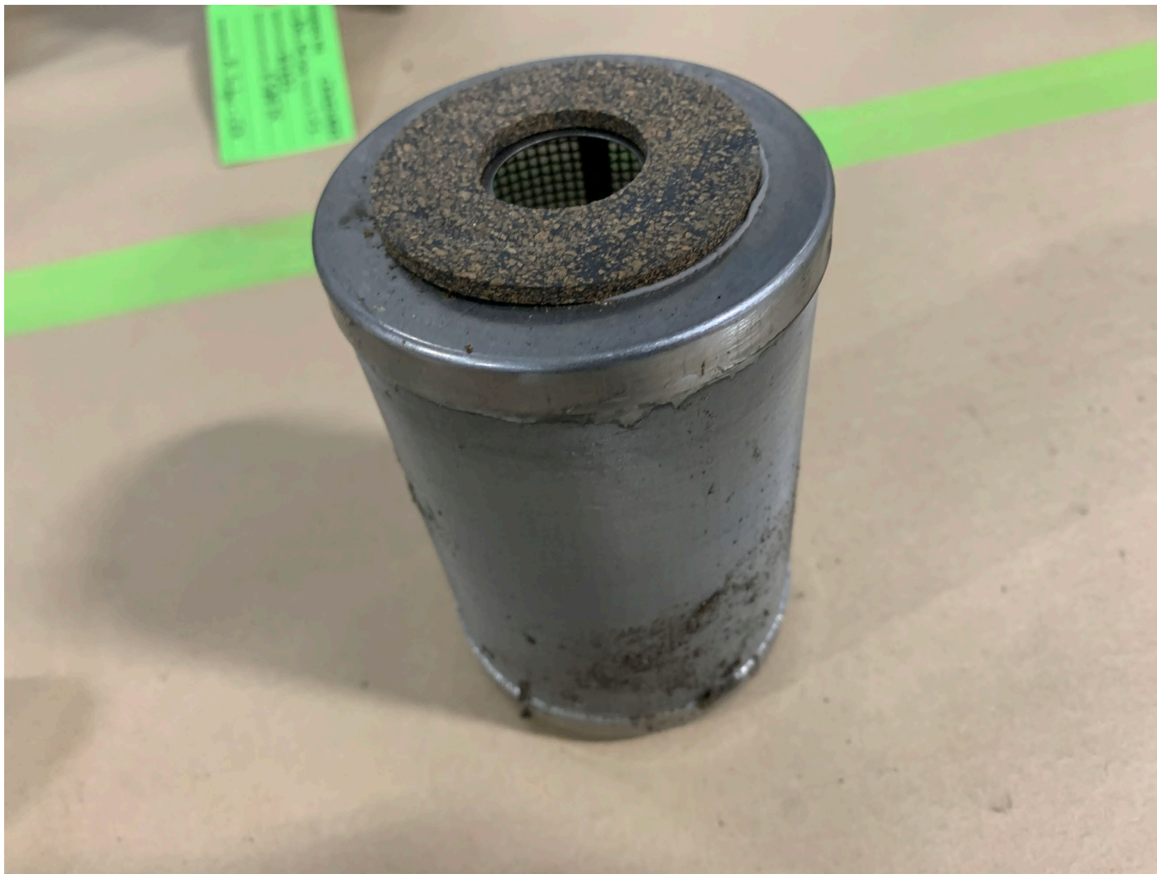
Photo 17 – View of the firewall fuel filter, with contamination.
