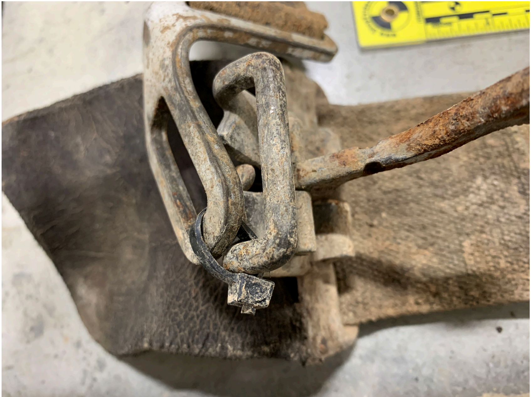
Photo 7 – View of a black zip tie, securing the left shoulder harness to the buckle assembly.
