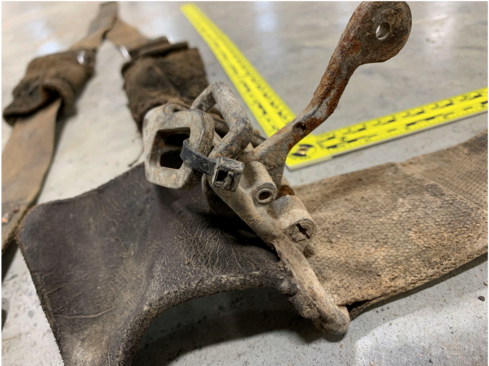
Photo 6 – View of a black zip tie, securing the left shoulder hardness to the buckle assembly.
