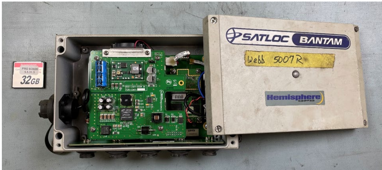
Figure 2. SATLOC M3 Bantam and internal CF card.
