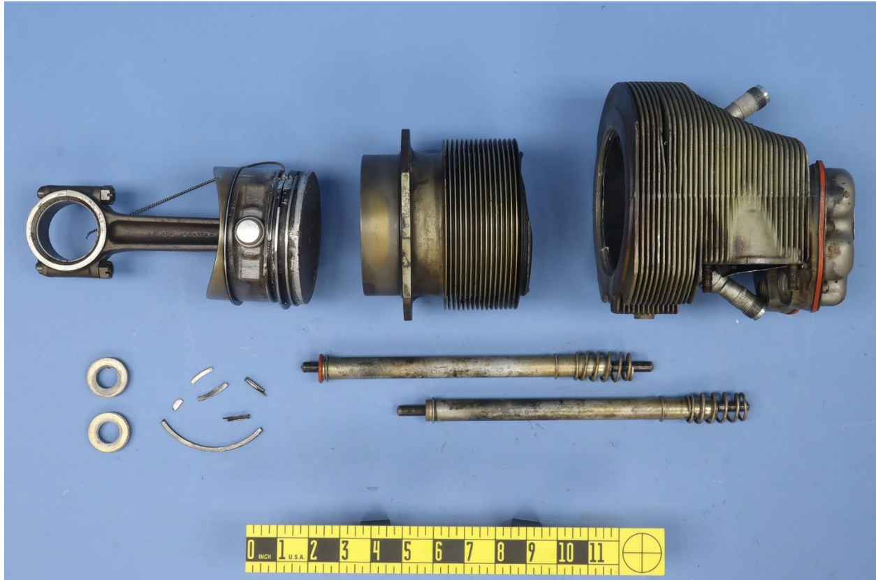
Figure 1. Fractured number three cylinder assembly and associated components, as received.
