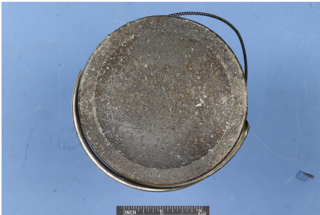
Figure 2. Number 3 piston crown exhibiting light pitting and impact damage.
