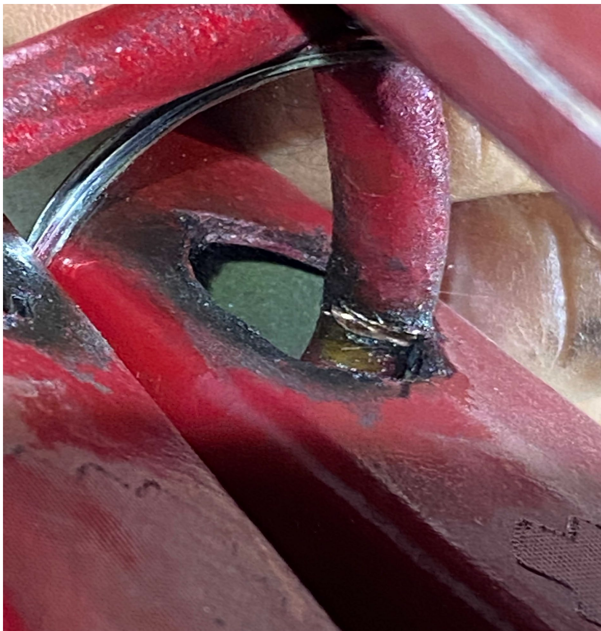
Photo 2 – Brake Line Damage Adjacent to the Cutout Hole in the Metal Support Bulkhead (Source: FAA)
